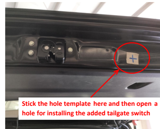
29. Stick the hole template to the tailgate as shown above and open a hole for installing the added tailgate switch.
