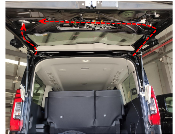
11. Route the left and right strut wiring harnesses to the tailgate.
