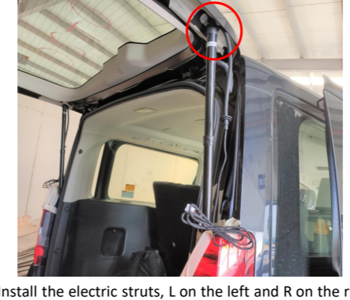
9. Install the electric struts, L on the left and R on the right (the first letter of the strut code), making sure the ends with wiring harnesses are on the tailgate.
