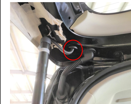
10. Thread the strut wiring harness through the circled hole. Both sides are the same
