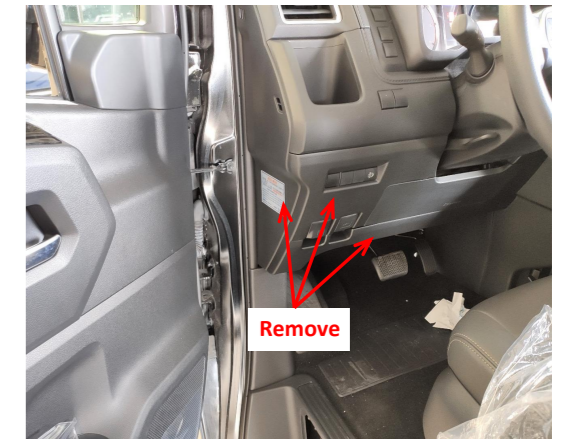
1. Remove the front left side trim panel and switch panel.
