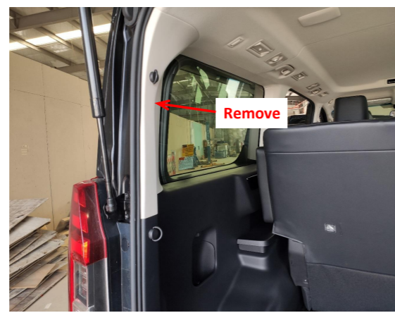
3. Remove the indicated trim panel to allow wiring harnesses to pass through.
