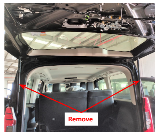
4. Remove the the original gas struts.
