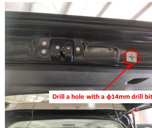
30. Drill a hole at the indicated position with a φ14mm drill bit.
