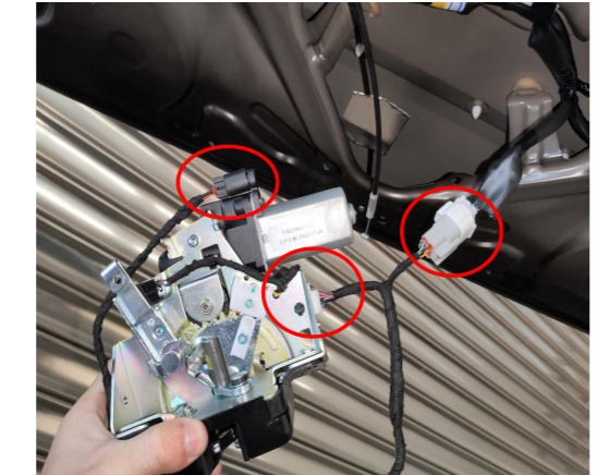
13. Connect the lock signal harness to the plugs of the power latch.
