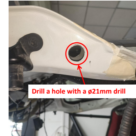
15. Use a \varnothing 21\text{mm} drill bit to drill a hole through two layers at the indicated position. Both sides are the same.
