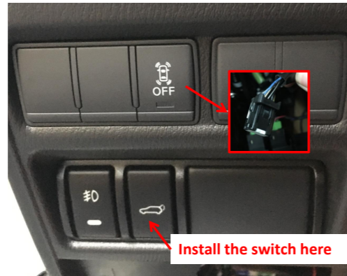
23. Install the switch at the indicated position. The small illustration shows the connection between the signal connector of backlight and our wiring harness connector.
