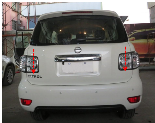
28. Initialize the system once, and then test each function of the electric tailgate.
