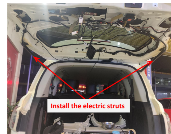
14. Install the electric struts, L on the left and R on the right (the first letter of the strut code).
