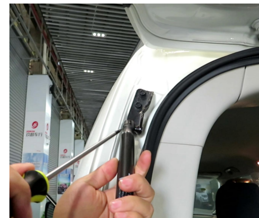
10. Remove the original gas struts.
