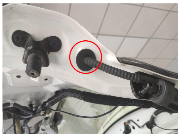
17. Thread the left and right strut wiring harnesses through the holes and plug the hole with rubber plugs.
