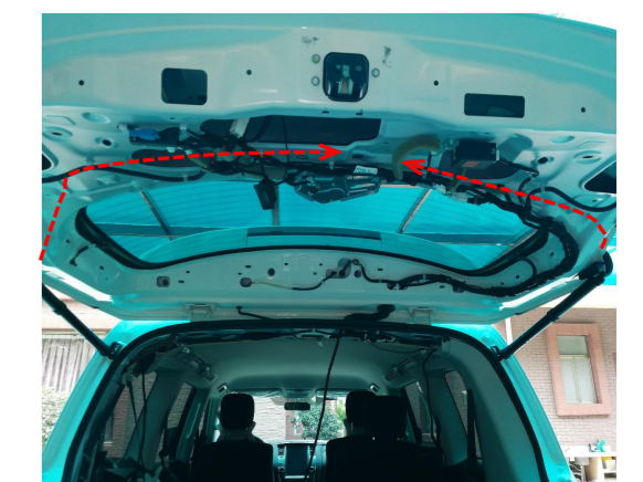
16. Route the strut wiring harnesses.
