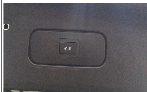
29. Reinstall all the trim panels and install the added tailgate switch at the tailgate handle.
