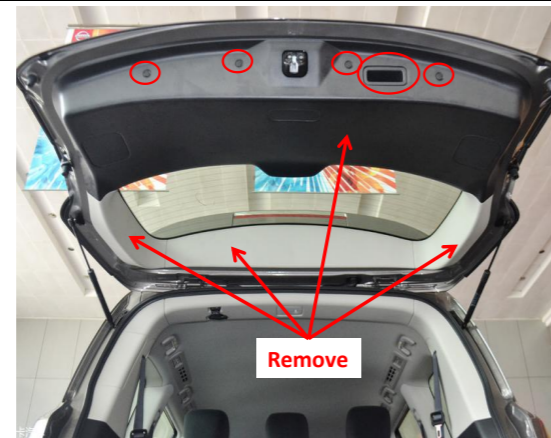
3. Remove the tailgate trim panels.
