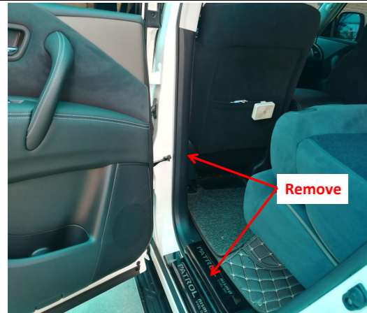
2. Remove the rear left side door sill trim panel and B-pillar trim panel.
