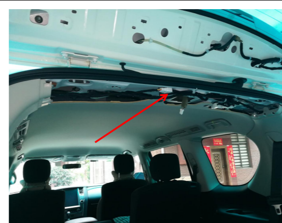
4. Remove the trunk roof trim panel.
