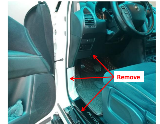
1. Remove the front left side trim panel, door sill trim panel and the exterior trim panel of fuse box.
