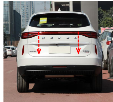
28. Press the added tailgate switch button to open and close the tailgate once for initializing the system, and then test the functions of the electric tailgate.
