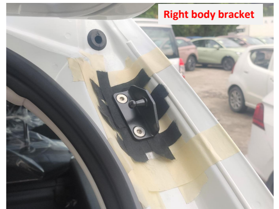
11. Replace the right body bracket.
