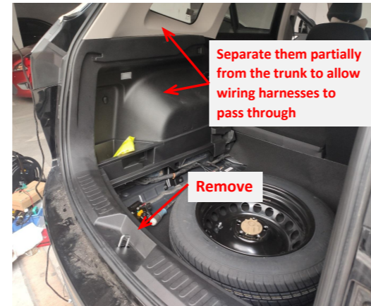
4. Remove the trunk floor mat, foam storage box, door sill panel and the trim panel on the left side of the trunk.
