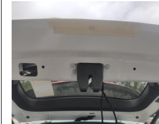
5. Remove the original latch and install our power latch.
