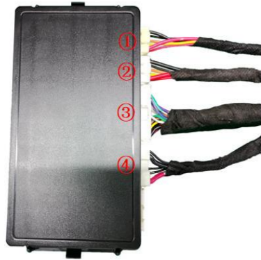
27. Insert the strut wiring harnesses ①②, lock signal harness ③, and power harness ④ into the ECU in sequence.
