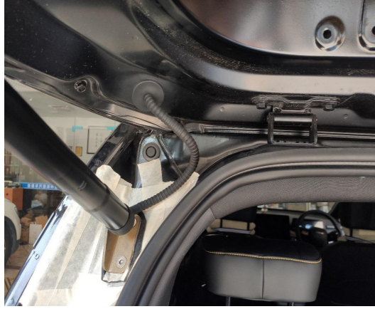
17. Plug the hole securely.
