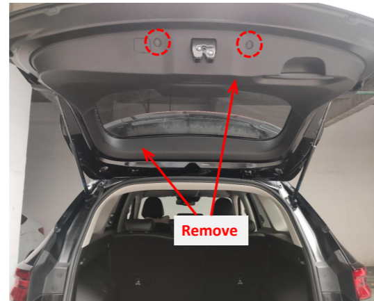
3. Remove the tailgate trim panels.
