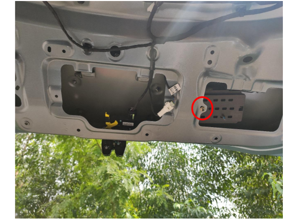
26. Fix the ECU at the indicated hole.
