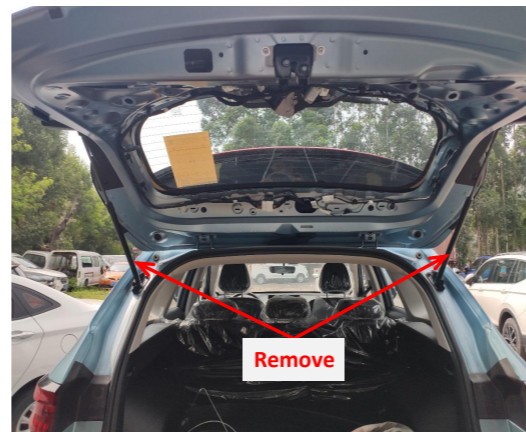
9. Remove the gas struts.
