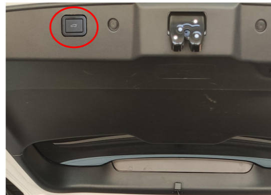
29. Reinstall all trim panels and install the added tailgate switch (remove the original small cover panel).
