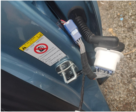
22. Connect the power harness to the B-pillar plugs at the rear left side B-pillar.
