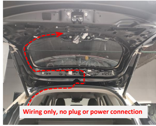
18. Route the power harness to the tailgate.
