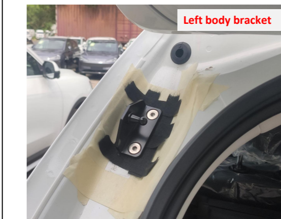
10. Replace the left body bracket.
