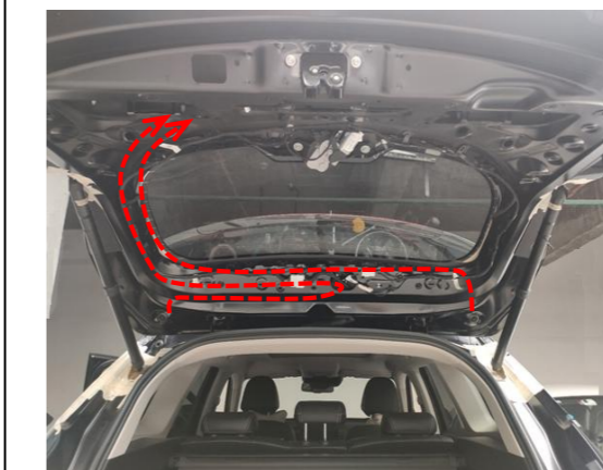
15. Route the strut wiring harness to the tailgate as shown above.
