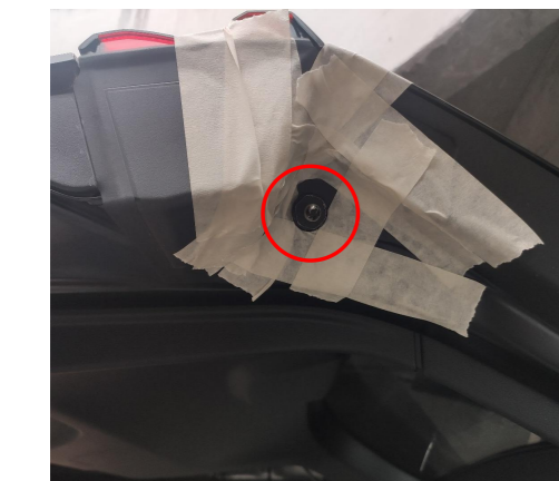
12. Replace the ball studs on both sides of the tailgate.
