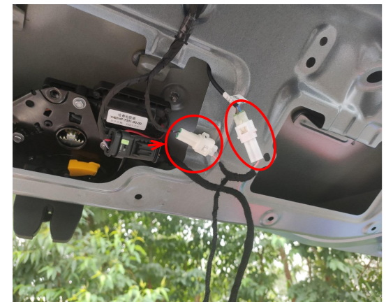
7. Connect the lock signal harness to the plugs of the original tailgate switch
