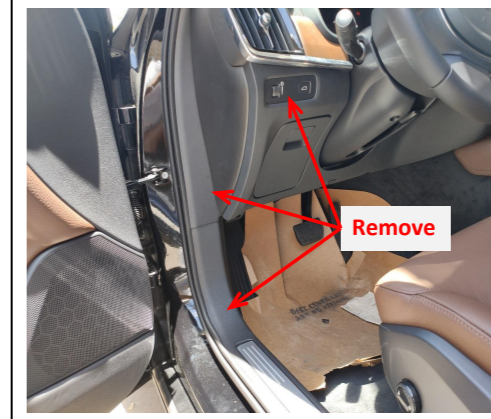
1. Remove the indicated trim panels, door sill panel and the tailgate switch button.
