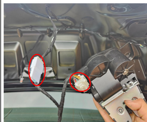
17. Connect the plugs of the lock signal harness to the plugs of the power latch.
