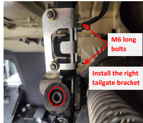
10. Install the right tailgate bracket. Secure the rubber cylinder head screw at the bump stop position and thread the M6 bolts from the inner side to the other side.
