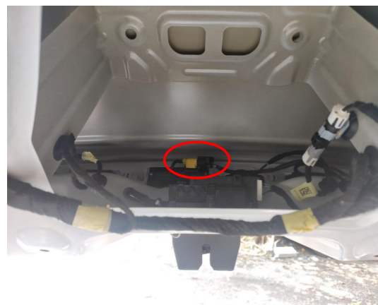
12. Connect the lock signal harness to the plug of original tailgate switch.
