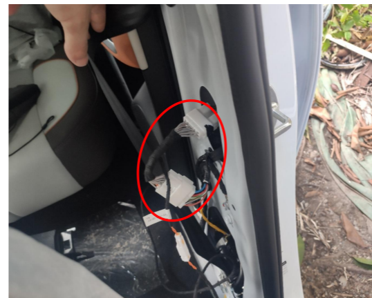
19. Connect the power harness to the B-pillar plugs at rear left side B-pillar.
