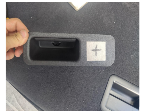
26. Stick the hole template to the indicated position of the handle and open a hole for the added tailgate switch.
