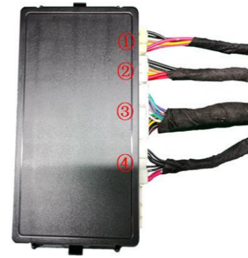
24. Insert the strut wiring harnesses ①②, lock signal harness ③, and power harness ④ into the ECU in sequence.
