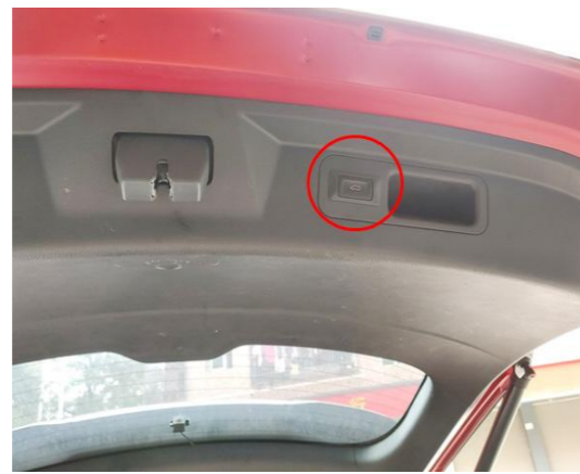
28. Reinstall all trim panels and install the added tailgate switch.
