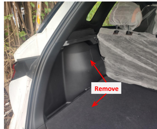
4. Remove the trunk floor mat and left side trim panel.
