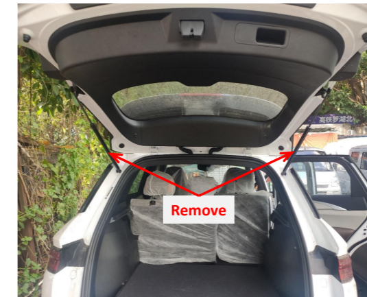
5. Remove the gas struts.
