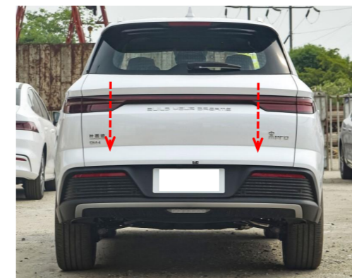
25. Press the added tailgate switch button to open and close the tailgate once for initializing the system, and then test each function of the electric tailgate.
