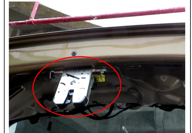
6. Remove the original latch and install our latch.
