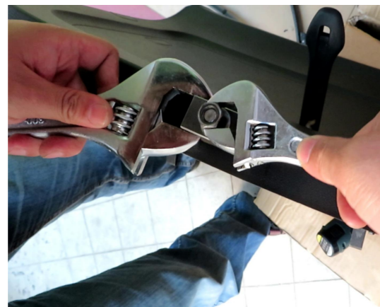
28. Open the hole (one hand holds the hole opener, the other turns the nut).
