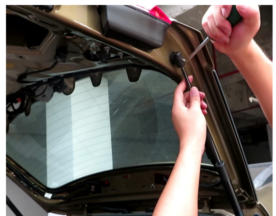
12. Remove the gas struts.
