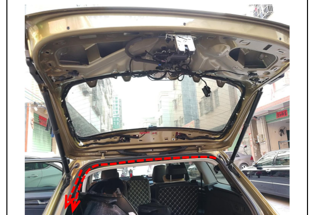
16. Route the strut wiring harnesses.
