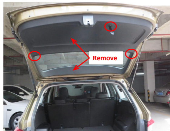
3. Remove the tailgate trim panels.
