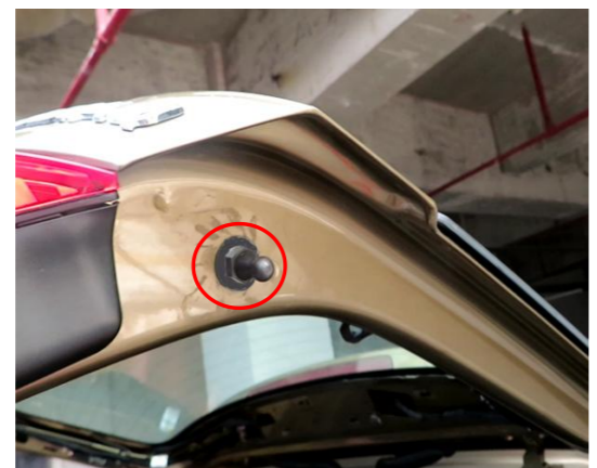
13. Install the provided ball stud.
