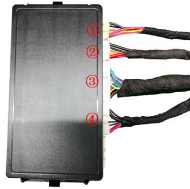
22. Insert the strut wiring harnesses ①②, lock signal harness ③, and power harness ④ into the ECU in sequence and mount the ECU onto its bracket.
