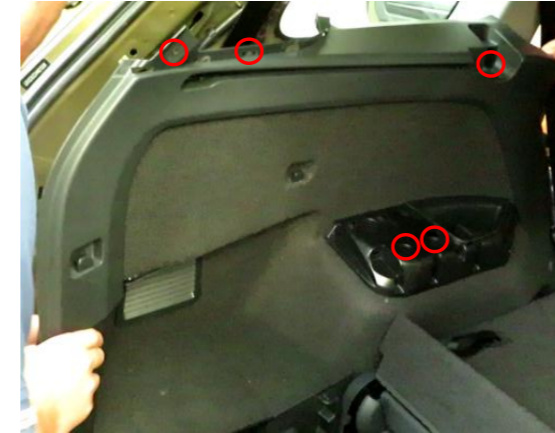
4. Remove the screws from left side trim panel of the trunk as shown above.
