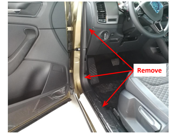
1. Remove the front left side trim panels and door sill panel.
