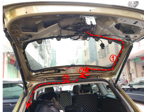
9. Route the lock signal harness to the trunk (do not insert terminals into the wiring harness connector for now).
