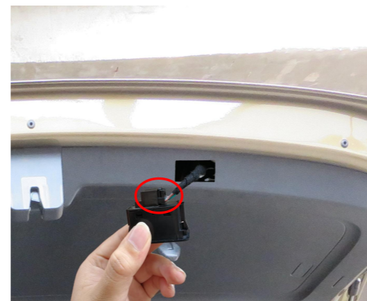
29. Reinstall all trim panels and fit the added tailgate switch in.
