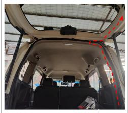
24. Thread the power harness to the tailgate routing only, no plug or power connection).
