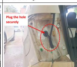
14. Wrap the wiring harness with electric tape and pay attention to avoid pulling it. Plug the holes on both sides securely.
