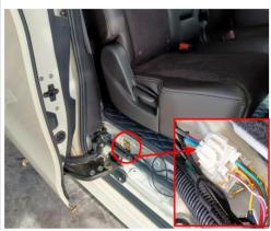
28. Connect the power harness to the indicated signal plugs at the rear right side door (the plug on the top).
