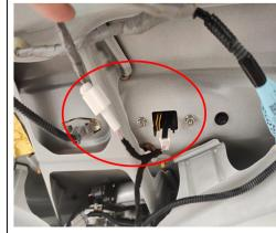
20. Connect the plugs of the lock signal harness to the plugs of the original tailgate switch.
