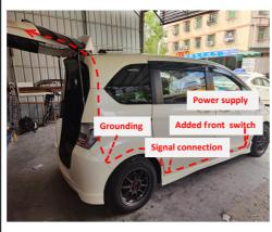
23. Route the power harness (routing only, no plug or power connection).
