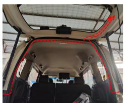
15. Route the strut wiring harnesses.
