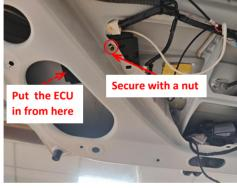
34. Install the ECU and secure it with a nut.
