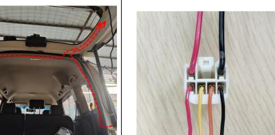
16. Insert the strut wiring harness terminals into the wiring harness connector.
