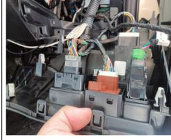
29. Install the added front switch and connect the 30. Check all the plugs. plugs for backlight.
