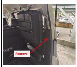
3. Remove the trim panel on the right side of the trunk to allow wiring harnesses to pass through.
