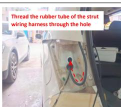
13. Thread the rubber tube of the strut wiring
