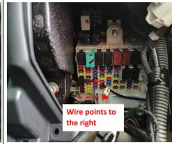
32. Plug the fuse tap into the fuse box and the pay attention to the direction.
