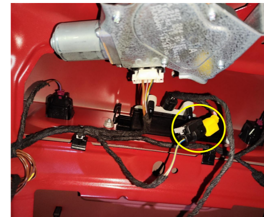
15. Connect the lock signal harness to the plugs of the original tailgate switch.
