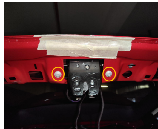
14. Install the power latch.
