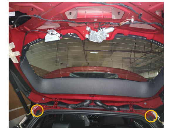
11. Plug the holes on both sides of the trunk securely.
