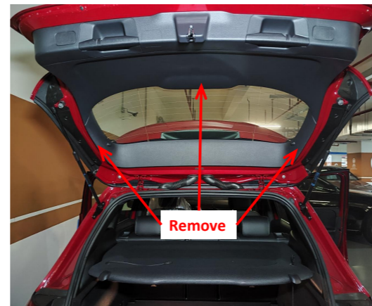
4. Remove the tailgate trim panels.
