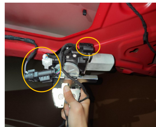
13. Remove the original latch and connect the lock signal harness with the plugs of the power latch.
