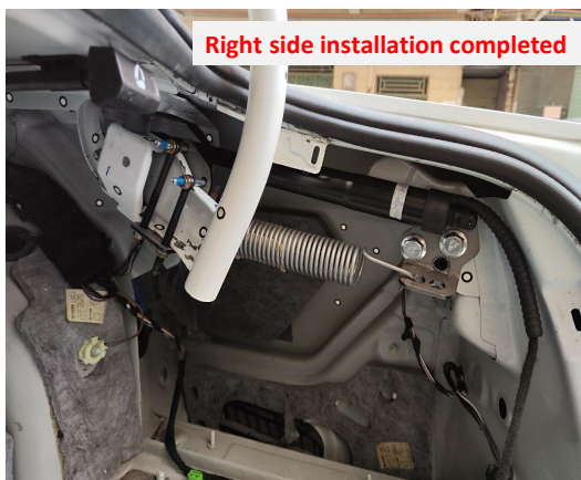
14. Route the right strut wiring harness to the left side of the trunk.
