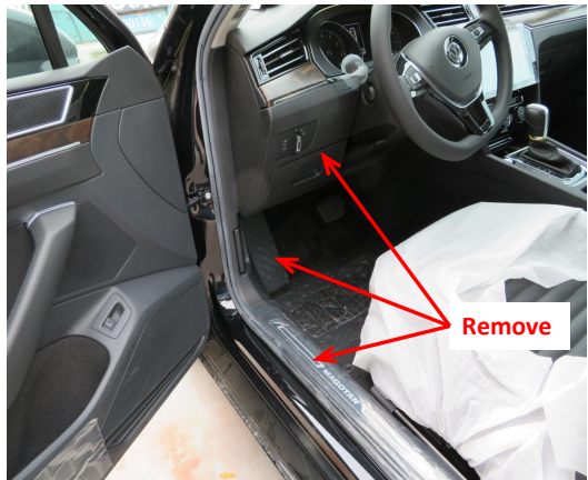
1. Remove the front left door sill trim, switch panel and the rest pedal.
