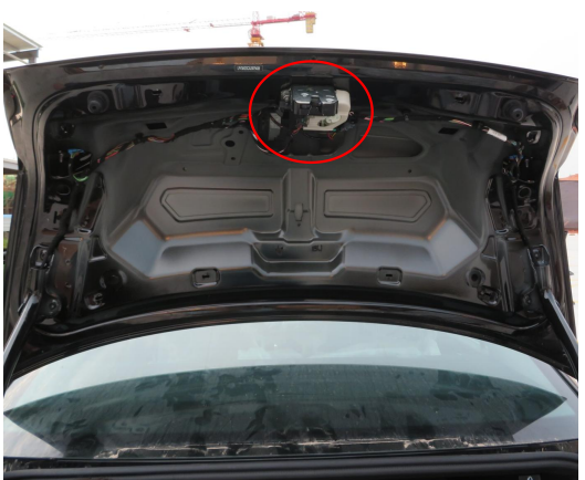
16. Connect the plugs of the lock signal harness to the power latch.
