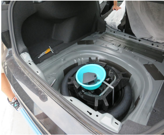
4. Remove the trunk floor mat and the door sill trim.
