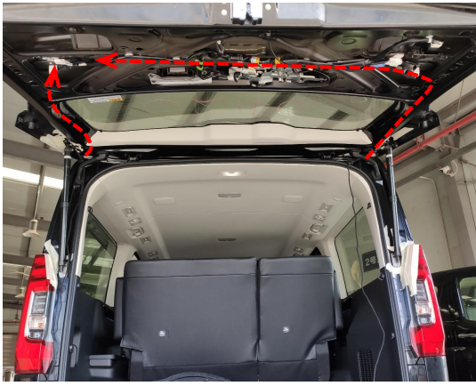
11. Route the left and right strut wiring harnesses to the tailgate.
