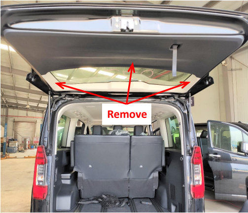
2. Remove the tailgate trim panels.
