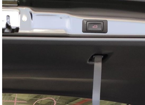
33. Install all the trim panels back and install the added tailgate switch.
