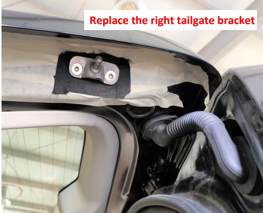
8. Replace the right tailgate bracket.
