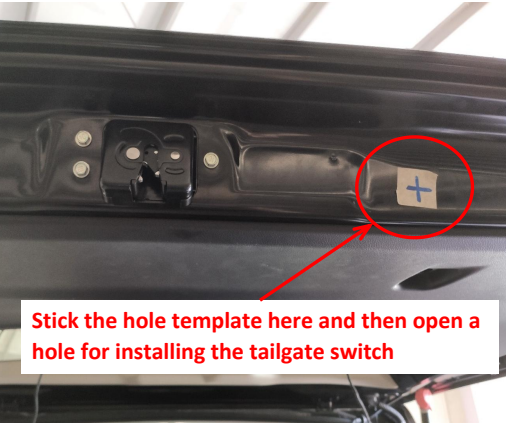
29. Stick the hole template to the indicated position of the tailgate and open a hole for installing the tailgate switch.
