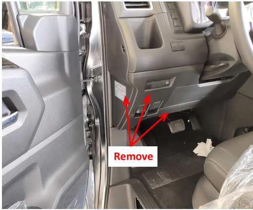
1. Remove the front left side trim panel and switch panel.
