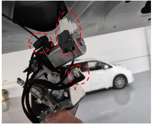
13. Connect the lock signal harness with the plugs of the power latch.
