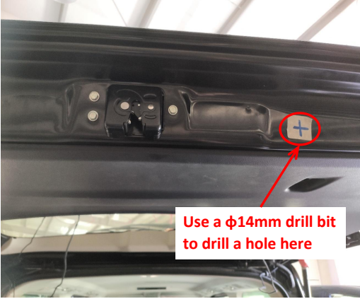
30. Drill a hole at the shown position of the tailgate using a \phi 14\text{mm} drill bit.
