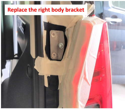
6. Replace the right body bracket.
