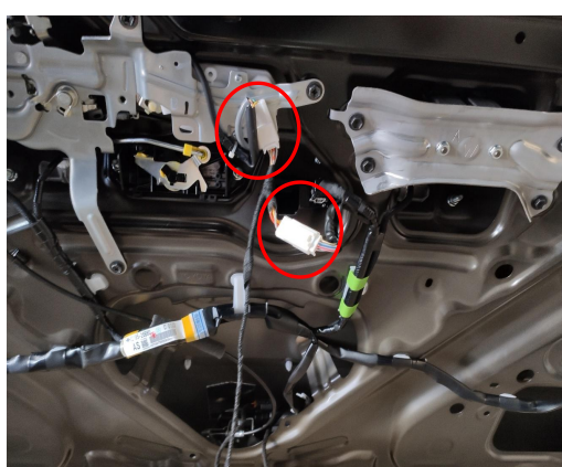
20. Connect the plugs of the power harness with the signal plugs at the tailgate.
