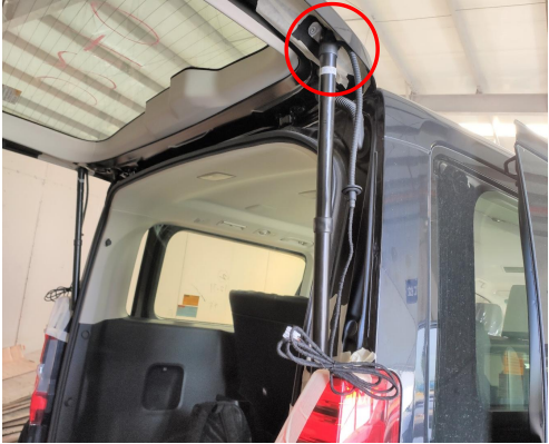
9. Install the electric struts, L on the left and R on the right (the first letter of the strut number), making sure the ends with wiring harnesses are on the tailgate.
