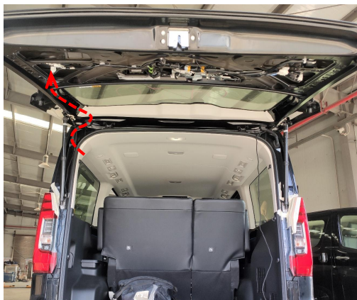
17. Thread the power harness to the tailgate (wiring only, no plug or power connection).
