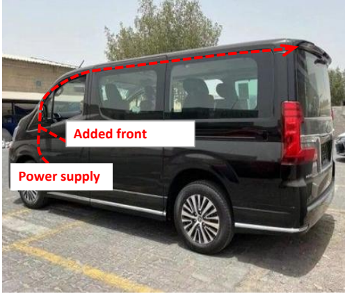
16. Route the power harness through the roof (routing only, no plug or power connection).
