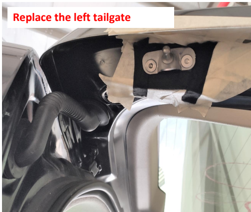
7. Replace the left tailgate bracket.
