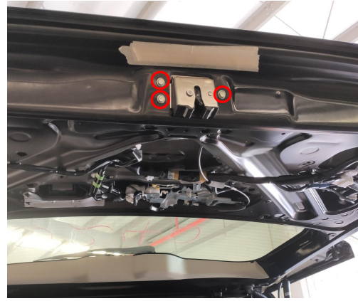
12. Remove the original latch.
