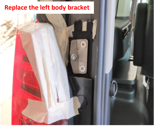
5. Replace the left body bracket.
