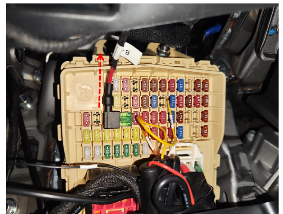
22. Plug the fuse tap into the fuse box and pay attention to the direction of wire.
