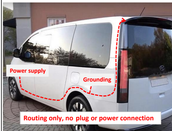
15. Route the power harness (if you need to install the added front switch, route the switch wiring harness in the same way).
