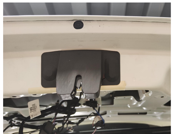
12. Install the power latch and cover the latch with the plastic casing.
