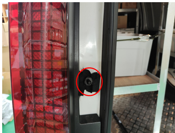
7. Replace the body ball studs on both sides of the trunk.
