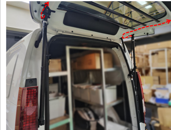
9. Thread the strut wiring harness through the holes in to the tailgate and route them as indicated.
