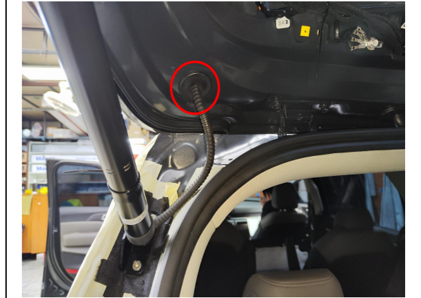
11. Plug the holes on both sides securely.
