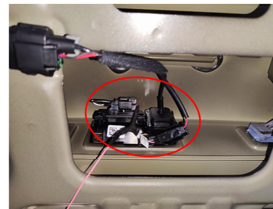
14. Connect the plugs of the lock signal harness to the plugs of original tailgate switch.
