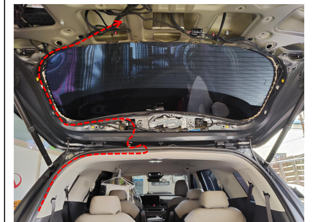
16. Thread the power harness to the tailgate.
