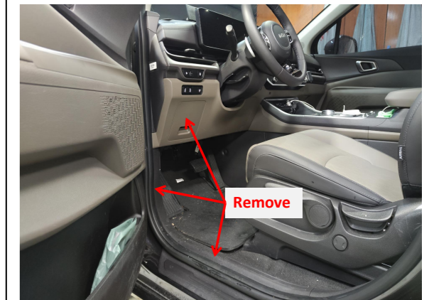
1. Remove the indicated front left side trim panel and door sill panels.
