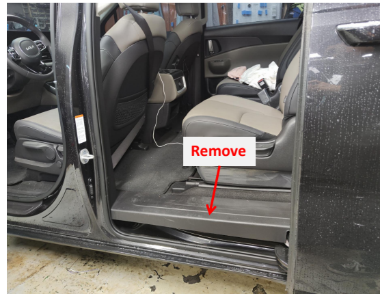
2. Remove the middle left step board.
