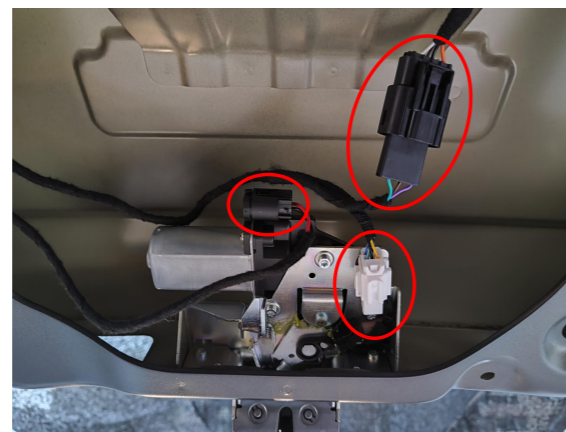
13. Connect the plugs of the lock signal harness to the plugs of the power latch.
