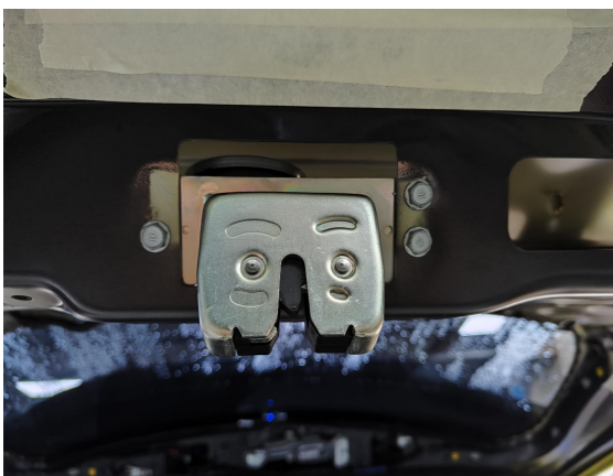
12. Remove the original latch and install the power latch.
