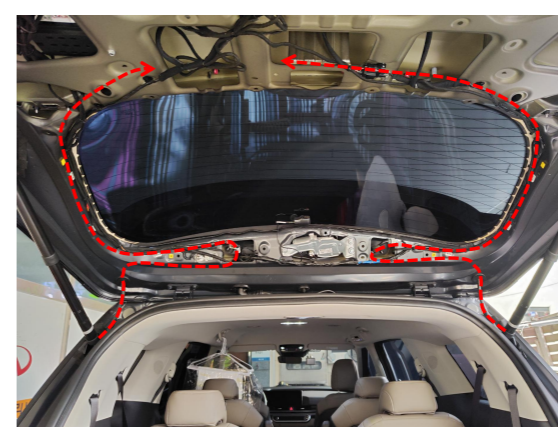
10. Thread the strut wiring harnesses through the holes on the tailgate and route the wiring harnesses as indicated.
