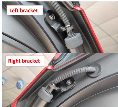
17. Replace the left and right tailgate brackets, and take care to differentiate between these two brackets.
