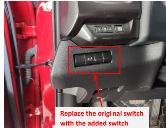
24. Replace the original switch with the added tailgate switch.
