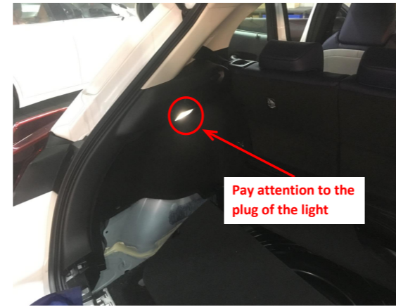
4. Remove the trim panel on the left side of the trunk.
