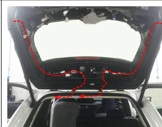
20. Thread the strut wiring harnesses through the tailgate to the left side of the trunk.
