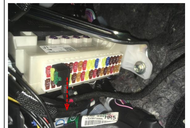
26. Plug the fuse tap into the fuse box with wire pointing downward.
