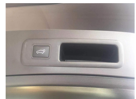
13. Install the added switch at the tailgate handle.
