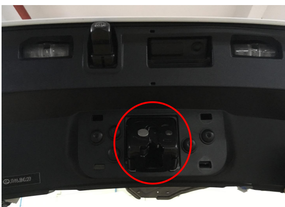
7. Insert the lock signal harness terminals into the wiring harness connector and then fasten the connector inward.
