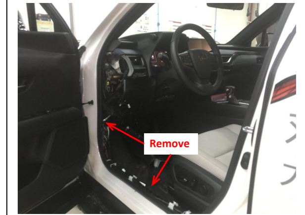
1. Remove the front left side trim panel and door sill panel.
