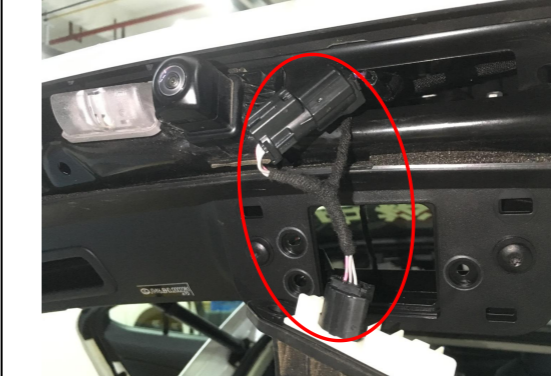
10. Connect the lock signal harness to the plugs of tailgate switch (choose the proper pair of plugs according to different models).
