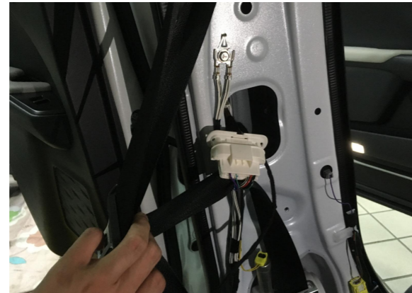
23. Connect the plugs of the power harness to the B-pillar plugs.
