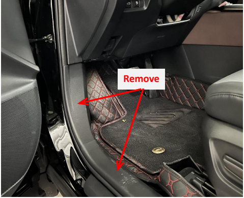
1. Remove the front left door sill panels.
