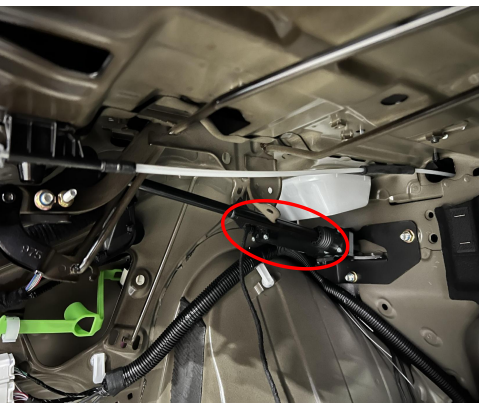
13. Install the left strut (L&R are marked as the first letter of the strut code).
