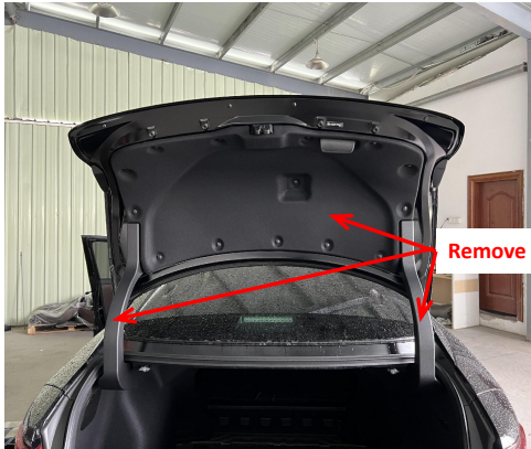
3. Remove the tailgate trim panel and hinge trim panels.
