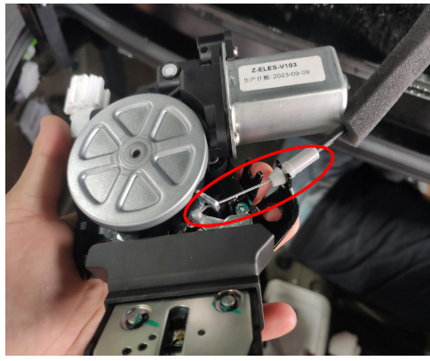
17. Install the original emergency cable onto the power latch (there are two fasteners. Choose the outer fastener)
