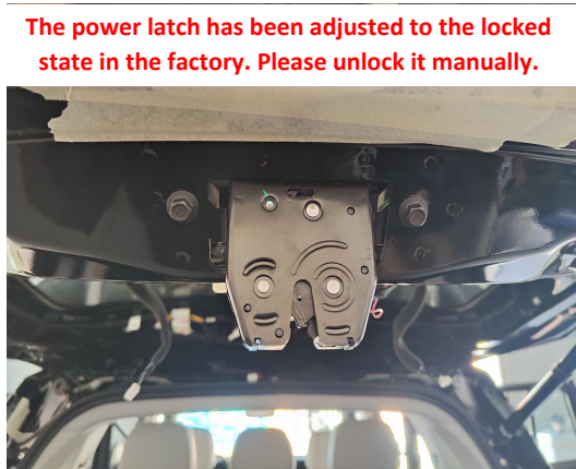
14. Install the power latch.(The original latch housing does not fit)
