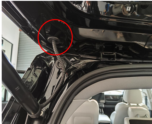
10. Pass the strut wiring harness through the indicated hole into the tailgate. Same on both sides.
