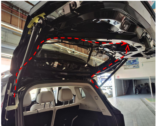
11. Route the left and right strut wiring harnesses as indicated and install the grommets.
