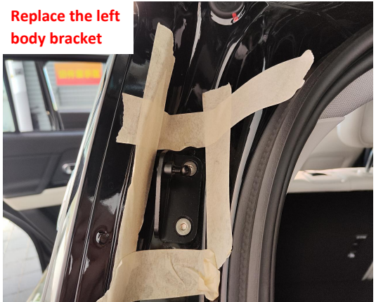
6. Replace the left body bracket.
