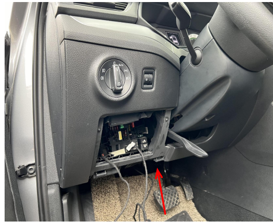
17. The CAN signal plug is located behind the steering column.
