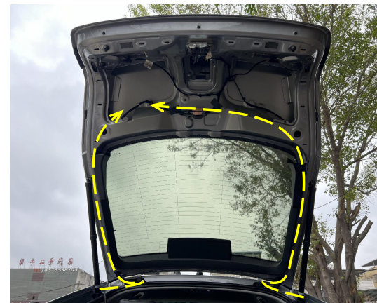
13. Thread the strut wiring harnesses into the tailgate and route them as indicated above.
