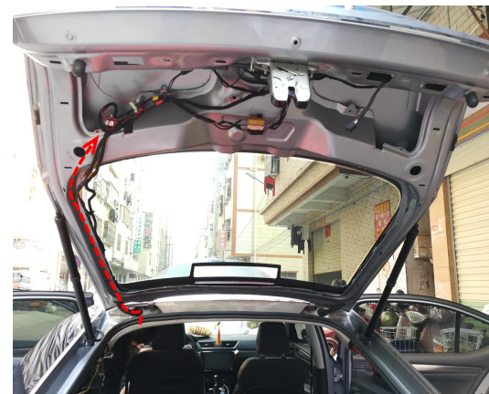
14. Thread the power harness into the tailgate and route it as indicated above.
