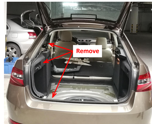
4. Take out the trunk floor mat and remove the indicated trim panels from the trunk.
