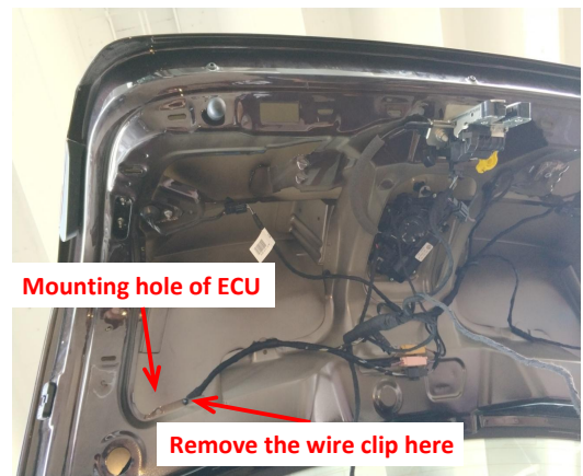
22. Locate the mounting hole of ECU.
