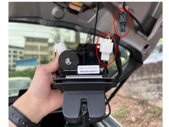
6. Put the plastic casing on the latch part and connect the plugs of the lock signal harness to the power latch.
