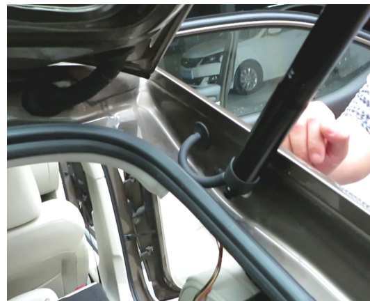
12. Install the electric struts, L on the left and R on the right (the first letter of the strut code).
