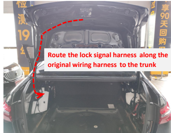
23. Route the lock signal harness to the trunk.
