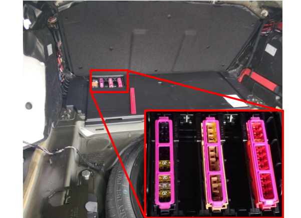
26. Connect to the fuse box for power supply (all the vacant slots are constant power).
