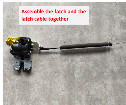
18. Assemble the latch and the latch cable together.
