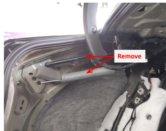
3. Remove the gas strut and the spring from the left side of the trunk.
