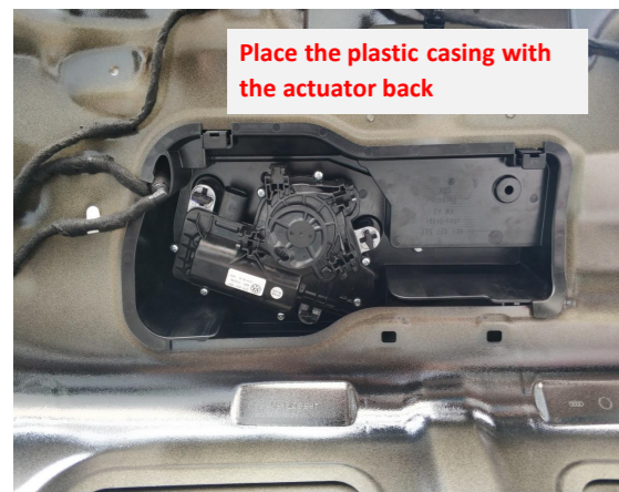
17. Place the plastic casing with the actuator back.
