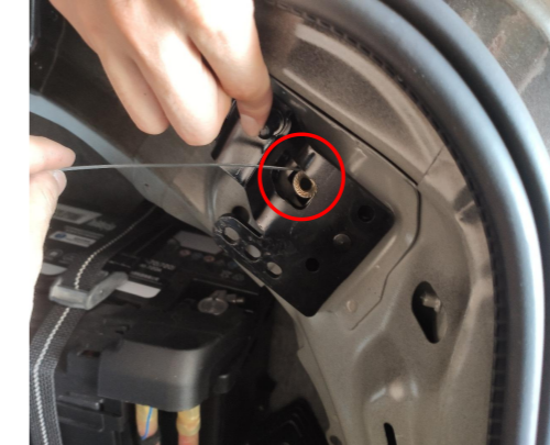
5. Install the right body bracket: insert the nut with handle into the indicated position, and secure it with a bolt.
