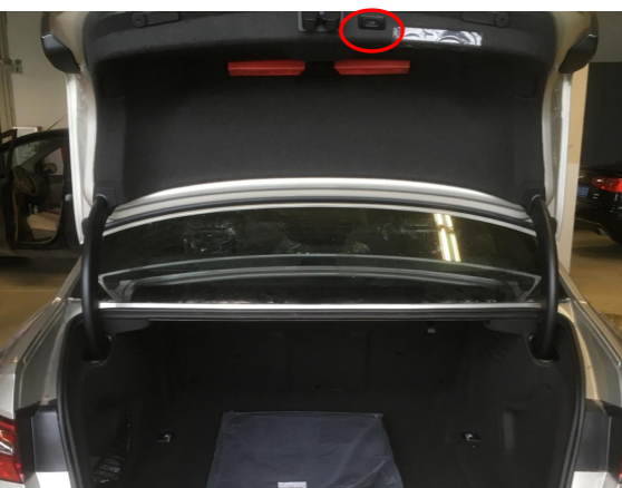
33. Reinstall all the trim panels and install the added tailgate switch.
