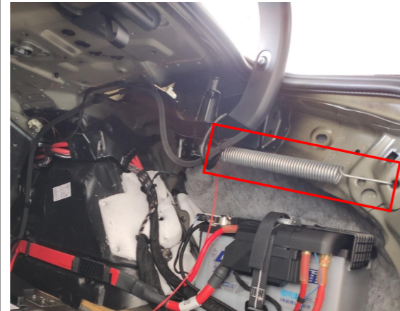
4. Remove the gas strut and the spring from the right side of the trunk.
