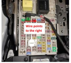
25. Plug the fuse tap into the fuse box. Pay attention to the direction.
