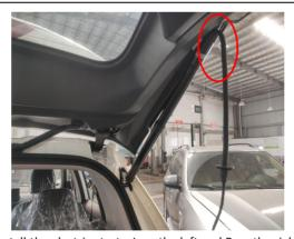
9. Install the electric struts, L on the left and R on the right the first letter of the strut code), making sure the ends with 10. Drill a hole at the indicated position with the  $\phi$ 21mm wiring harnesses are on the tailgate.
