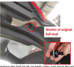
8. Replace the ball studs on both sides and place the original washers under them.
