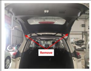
5. Remove the original gas struts. 6. Replace the bracket on the left side of the car body.
