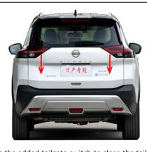
30. Press the added tailgate switch to close the tailgate, and open it to complete the system initialization. Then test each function of the electric tailgate.
