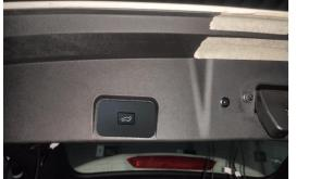
32. Install the added tailgate switch and reinstall all trim panels.
