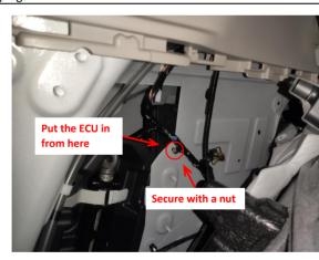
28. Install the ECU and secure it with nut.
