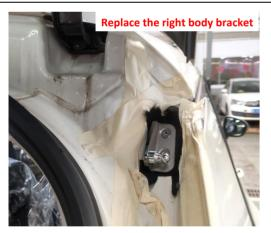
7. Replace the bracket on the right side of the car body.
