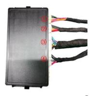
29. Insert the left and right strut wiring harnesses (1)(2), lock signal harness ③, and power harness ④ into the ECU in sequence.
