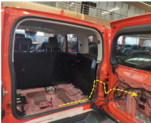
15. Route power harness to the tailgate (no plug connection before inserting terminals into wiring harness connector).
