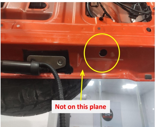
9. Drill a hole at the indicated position with a φ21mm drill bit to allow the strut wiring harness to pass through.
