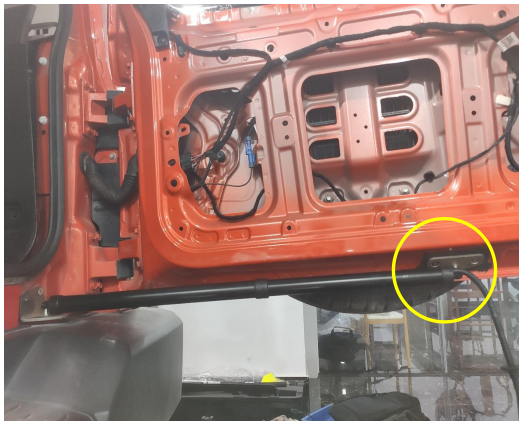
8. Install the electric strut, making sure the end with wiring harness is on the tailgate.
