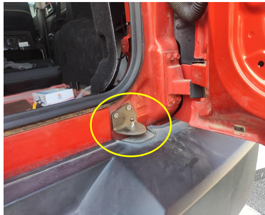
6. Replace the original body bracket.
