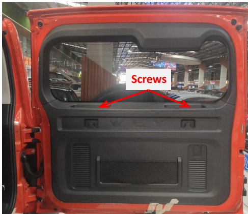
3. Remove the tailgate trim panels.
