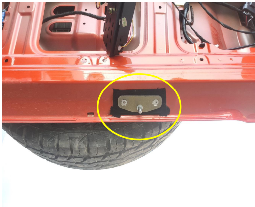
7. Replace the original tailgate bracket.
