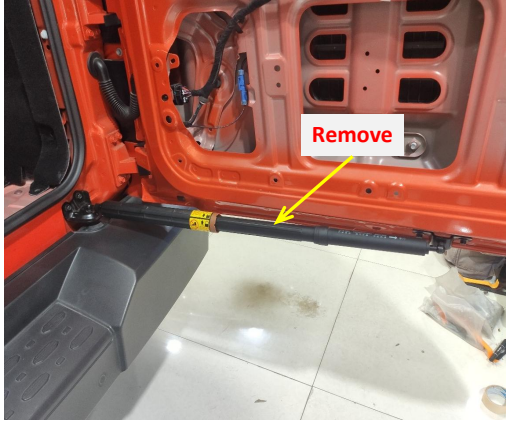
5. Remove the original gas strut.
