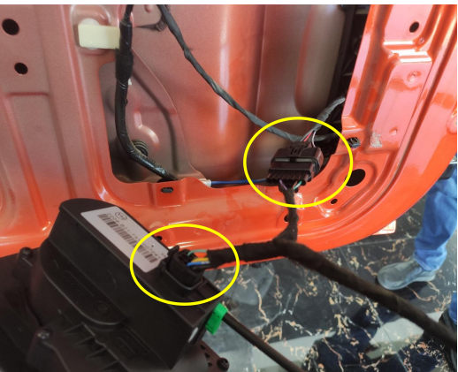
12. Connect the plugs of the lock signal harness to the power latch.
