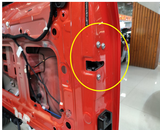
11. Remove the original latch.
