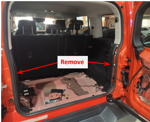
4. Take out the trunk floor mat and foam storage box. Remove the trim panels on both sides of the trunk.
