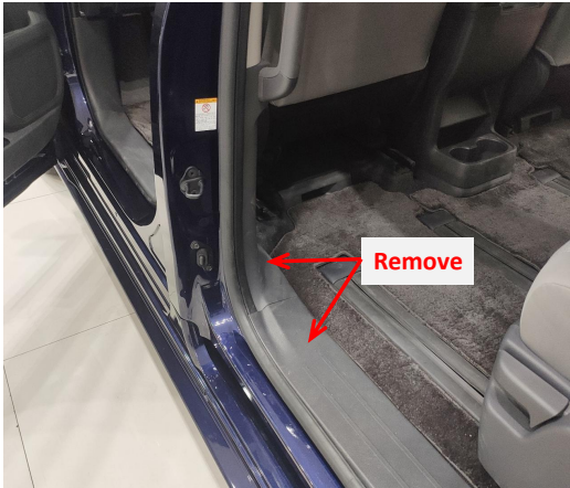
2. Remove the rear left door sill panel and B-pillar trim panel.
