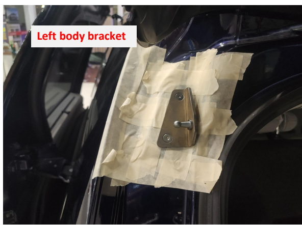
6. Replace the left body bracket.
