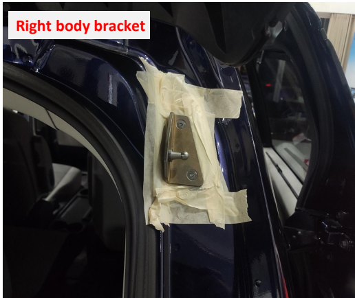
7. Replace the right body bracket.
