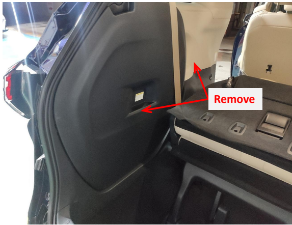
3. Remove the trim panels on the left side of the trunk.
