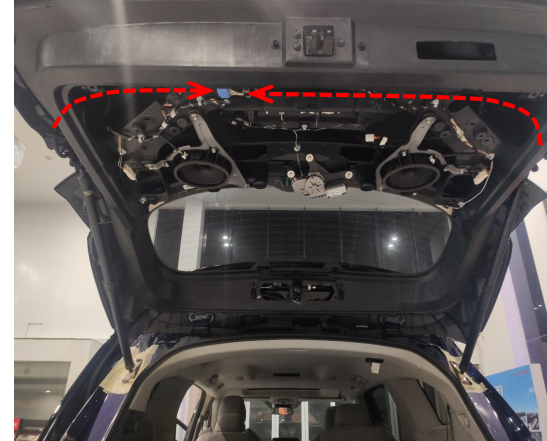
10. Route the strut wiring harnesses.
