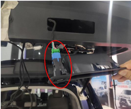
14. Connect the lock signal harness to the added tailgate switch.
