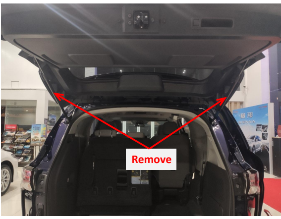
5. Remove the original gas struts.
