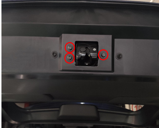
11. Replace the original latch with our power latch.
