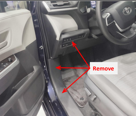
1. Remove the front left door sill panels, switch panel and storage box.
