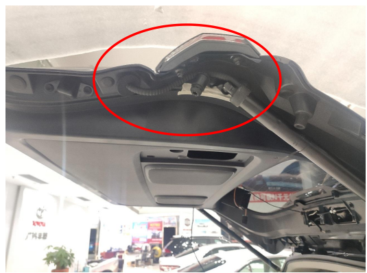
9. Thread the strut wiring harness through the original car hole into the tailgate, plug the hole tightly and then place the rubber tube between the bump stop and the tailgate.
