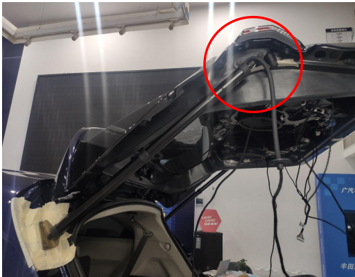
8. Install the electric struts, L on the left, R on the right(the first letter of the strut code), making sure the ends with wiring harnesses are on the tailgate.
