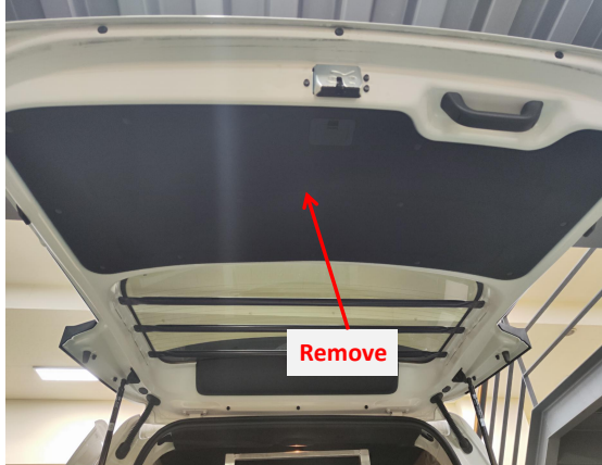
3. Remove the tailgate trim panel.
