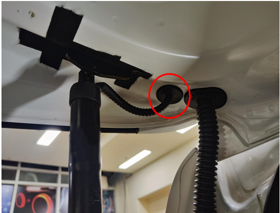
10. Plug the holes on both sides securely.
