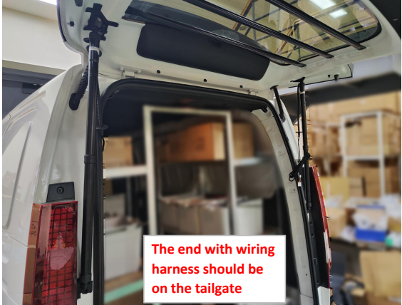
8. Install the electric struts, L on the left and R on the right (the first letter of the strut code).
