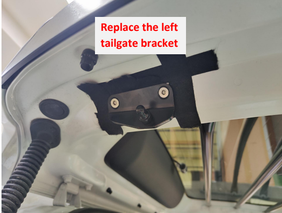
5. Replace the left tailgate bracket.
