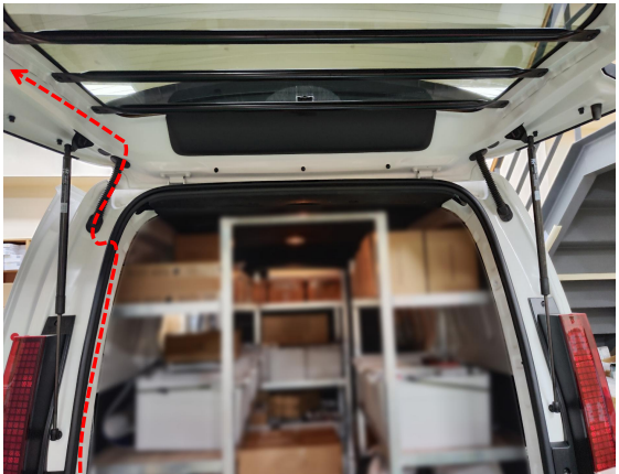
16. Thread the power harness to the tailgate.
