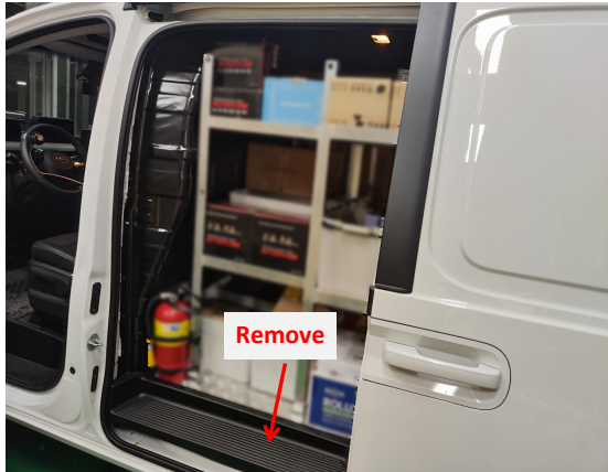
2. Remove the middle door step board.
