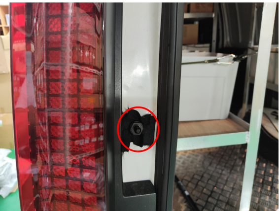
7. Replace the body ball studs on both sides of the trunk.
