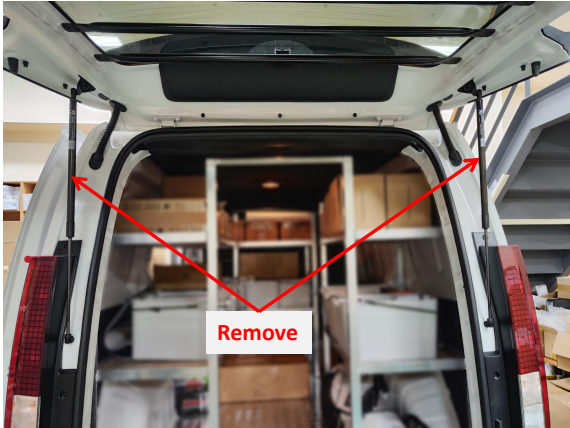
4. Remove the original gas struts.
