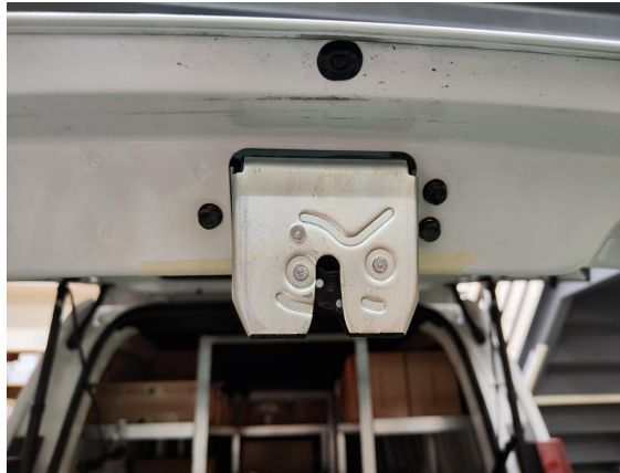
11. Remove the original latch.
