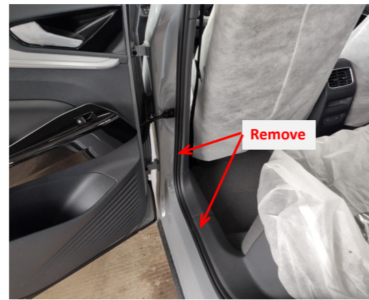
3. Remove the rear left side door sill panel and B-pillar trim panel.
