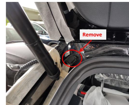
10. Remove the rubber plug from the hole to allow the strut wiring to pass through; both sides are the same.
