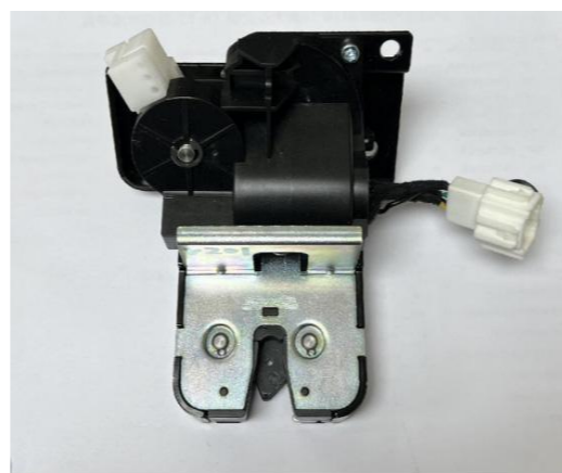
14. Remove the plastic housing from the power latch and cut off the cable tie.
