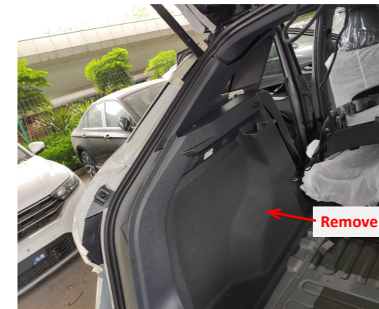
5. Remove the trim panel on the left side of the trunk.
