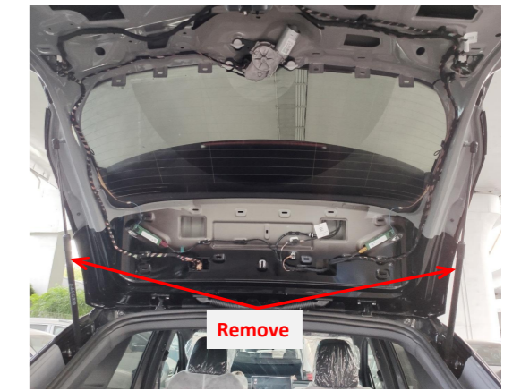
6. Remove the original gas struts.
