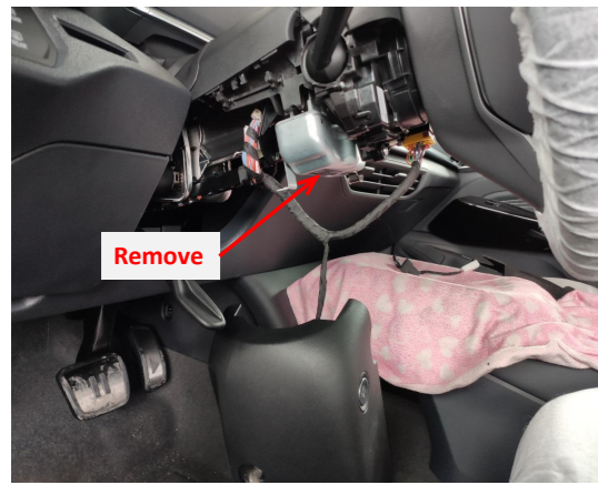
2. Remove the lower trim panel of the steering wheel.
