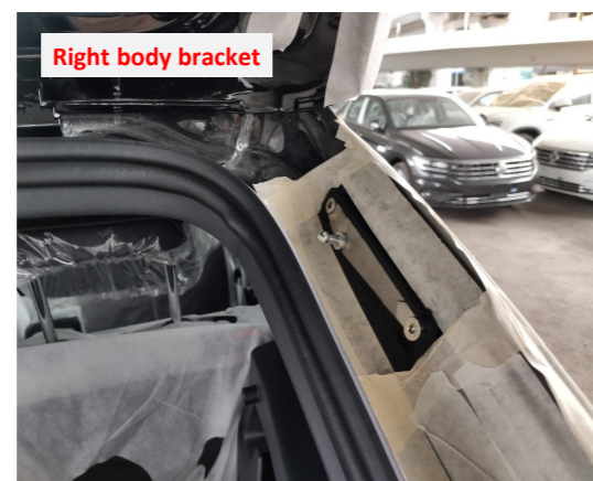
8. Replace the right body bracket.
