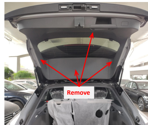
4. Remove the tailgate trim panels.
