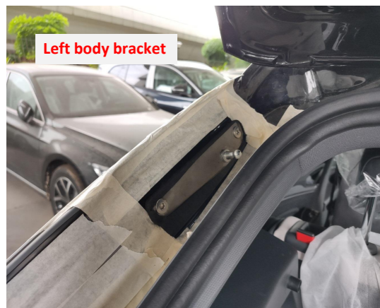
7. Replace the Left body bracket.
