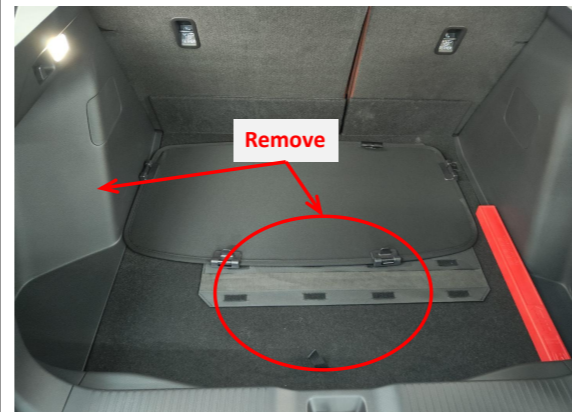
4. Remove the trunk floor mat and the trim panel on the left side of the trunk.
