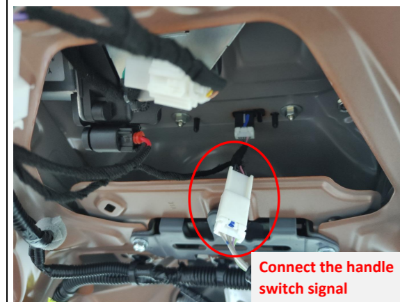
12. Connect the plugs of the lock signal harness to the plugs of the original switch.
