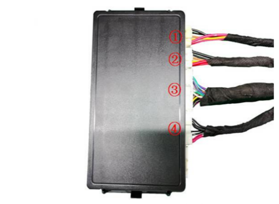
24. Insert the strut wiring harnesses ①②, lock signal harness ③, and power harness ④ into the ECU in sequence.
