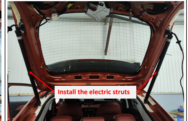
6. Install our electric struts.
