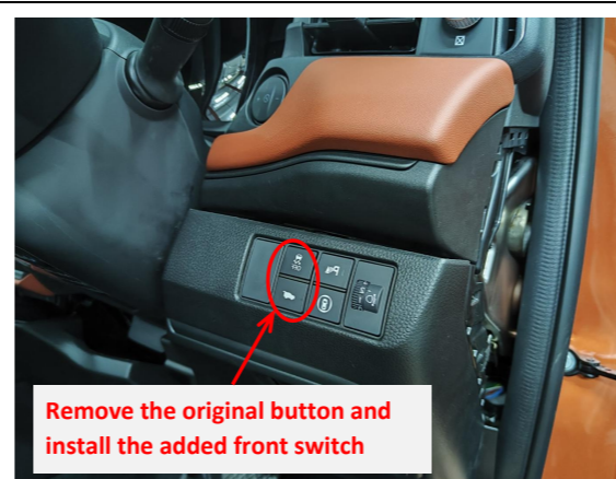
19. Remove the original button and install the added front switch.
