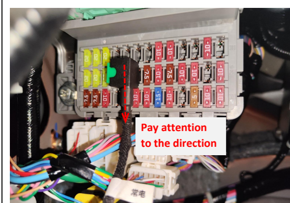
22. Plug the fuse tap into the fuse box and pay attention to the direction.
