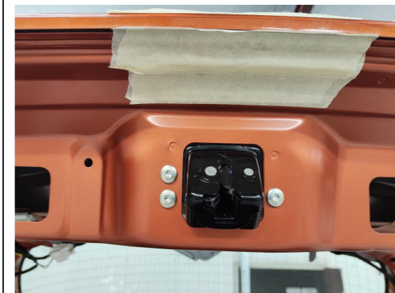
10. Remove the original latch.
