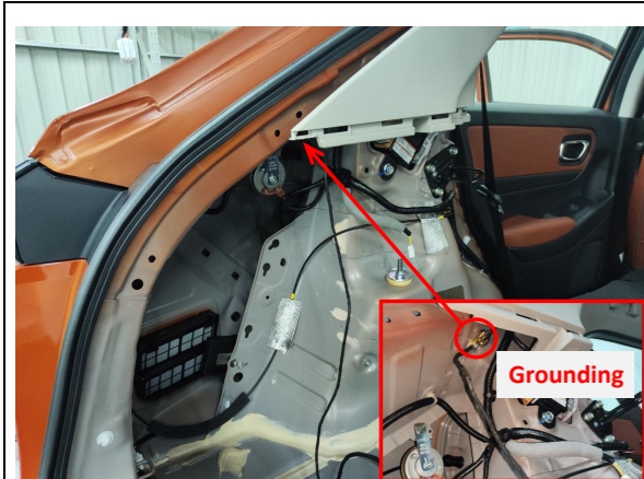
17. Ground at the left side of the trunk.
