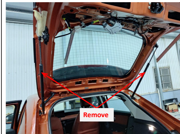
5. Remove the original gas struts.
