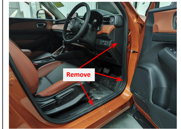
1. Remove the indicated driver side trim panels.
