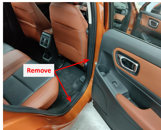
2. Remove the rear right side B-pillar trim panel and door sill panel.
