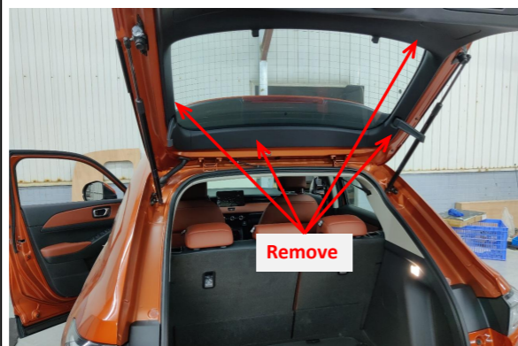
3. Remove the tailgate trim panels.
