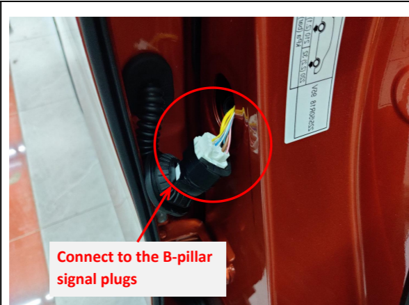
18. Connect the plugs of the power harness to the B-pillar signal plugs.
