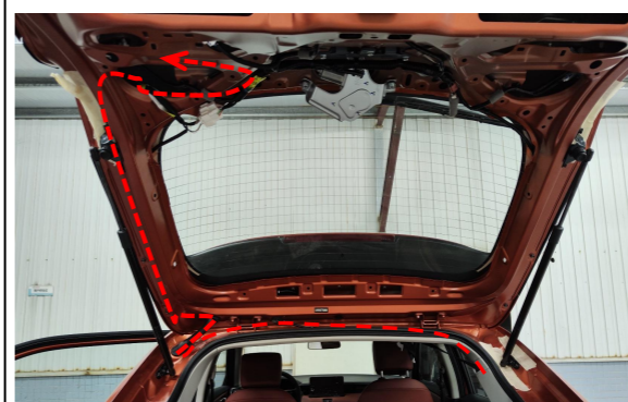
15. Thread the power harness to the tailgate as indicated.
