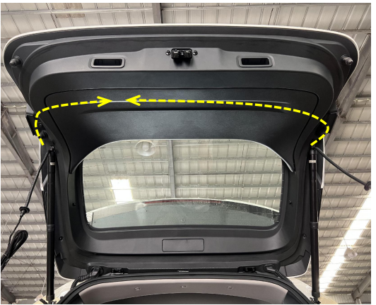
11. Route the strut wiring harnesses as indicated.
