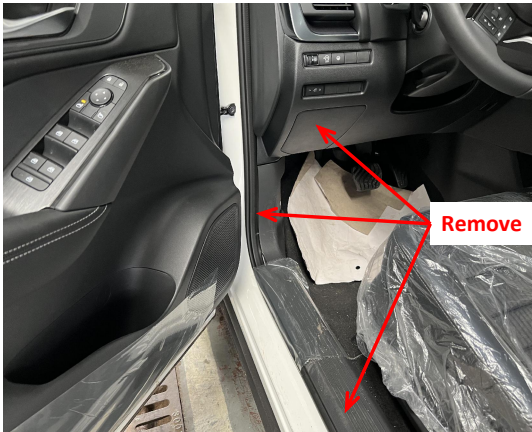
1. Remove the front left door sill panel and the trim panel of fuse box.
