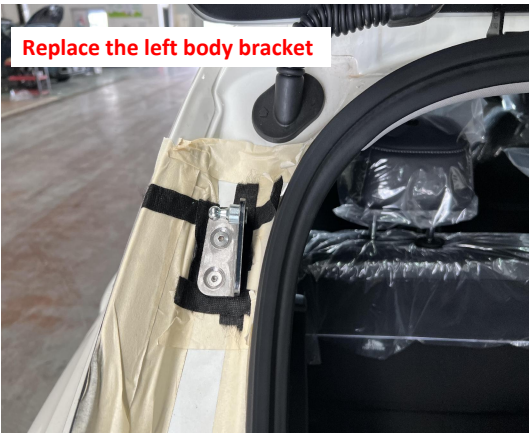
6. Replace the bracket on the left side of the vehicle body.
