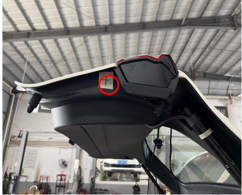
10. Drill a hole at the indicated location with a φ21mm drill bit to allow wiring harness to pass through, the same on the other side.
