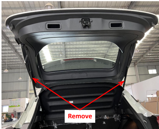
5. Remove the original gas struts.
