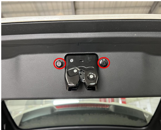
13. Remove the original latch.
