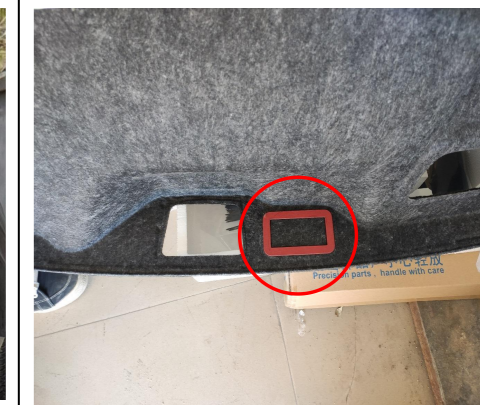
32. For model without the tailgate switch, stick the hole template to the indicated position and open a hole for the added tailgate switch.
