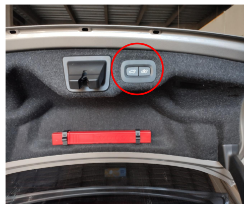
33. Fit the added tailgate switch in and reinstall all trim panels.
