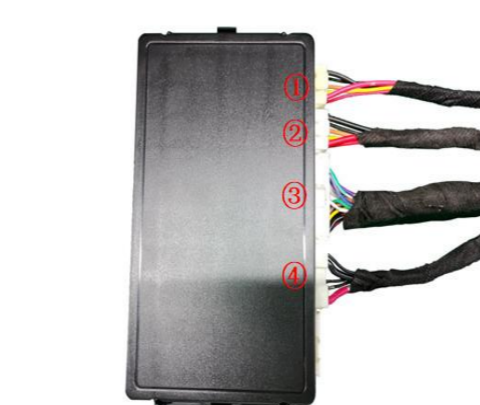
29. Insert the left and right strut wiring harnesses ①②, lock signal harness ③, and power harness ④ into the ECU in sequence.
