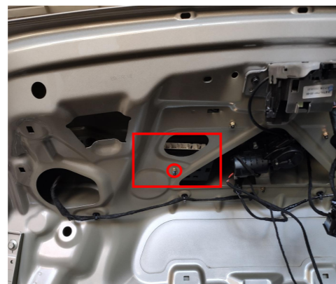
28. Secure the ECU bracket at the indicated position.
