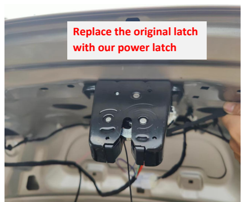
15. Remove the original latch and install our power latch.
