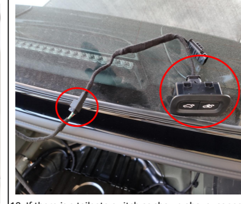
18. If there is a tailgate switch as shown above, connect it to the plug of lock signal harness. If there is no such tailgate switch, connect the provided tailgate switch to the plug of lock signal harness.
