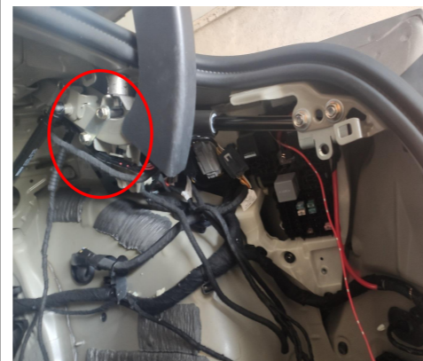
11. Install the electric struts, L on the left and R on the right (the first letter of the strut code). The end with wiring harness should be on the hinge.
