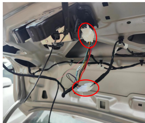
16. Connect the plugs of the lock signal harness to the plugs of power latch.
