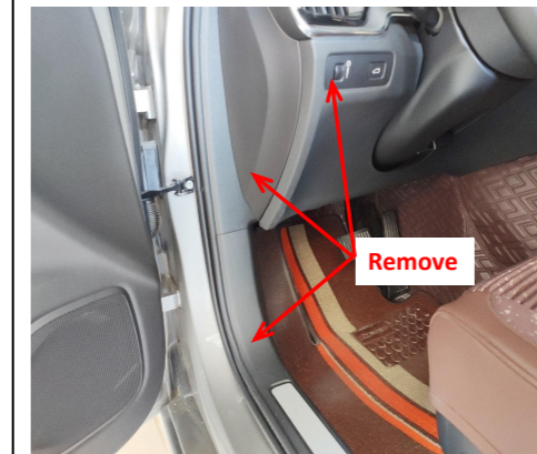
1. Remove the indicated driver side trim panels and door sill panel.
