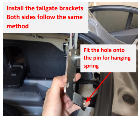
9. Install the tailgate brackets. Both sides follow the same method.
