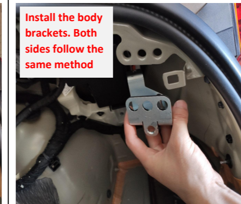
6. Install the body brackets. Both sides follow the same method.
