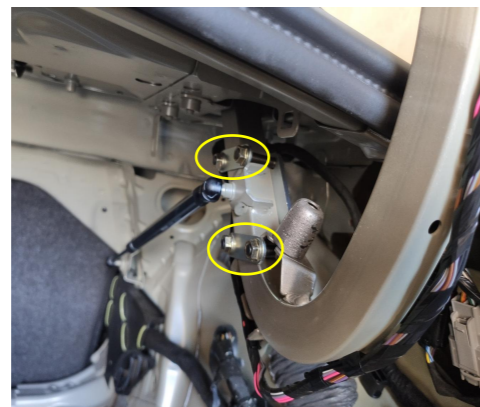
10. Secure the tailgate bracket with the bolts and shims.
