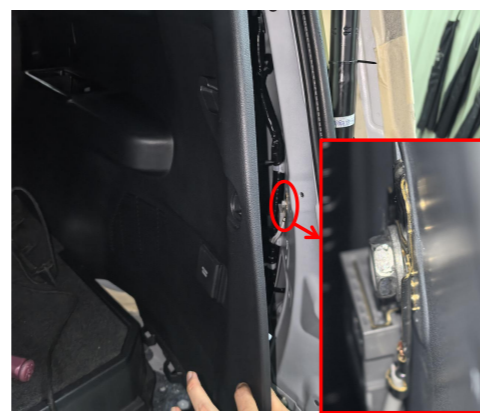
23. Ground at the indicated position on the right side of the trunk.
