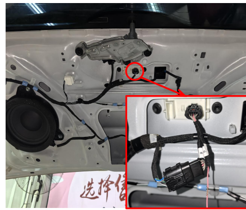
21. Connect the plugs of the lock signal harness to the plugs of original tailgate switch.
