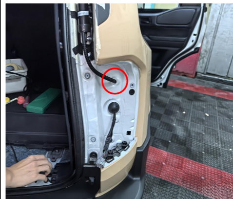
12. Remove the upper hole plug and thread the strut wiring harness through that hole into the body.
