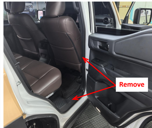
3. Remove the indicated rear right side door sill panel and B-pillar trim panel.
