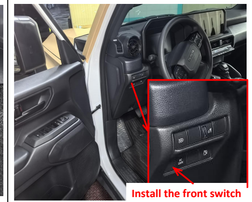
26. Remove the blank button from the switch panel and install the added front switch.
