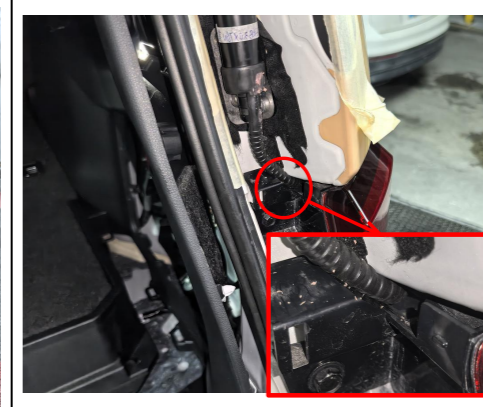
13. Reinstall the taillights and pay attention to the position of the strut wiring harness.
