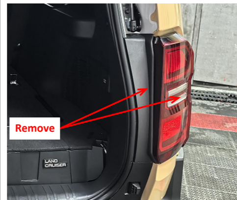
11. Remove the taillights on both sides.
