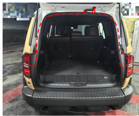
15. Route the left and right strut wiring harness to the tailgate as indicated.
