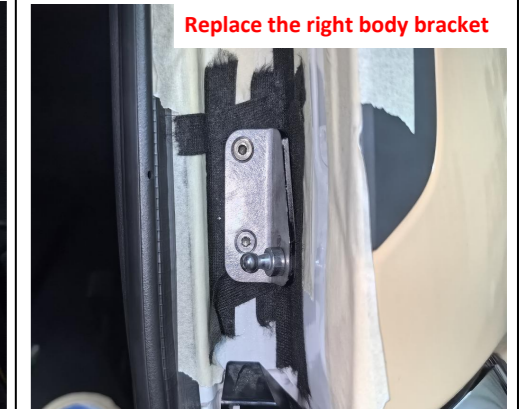
8. Replace the right body bracket.
