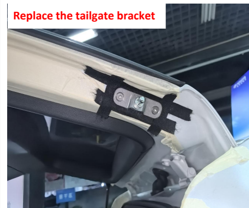
9. Replace the tailgate brackets on both sides of the tailgate.
