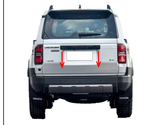
37. Press the added tailgate switch to close the tailgate once, the system completes initialization, and then test each function of the electric tailgate.
