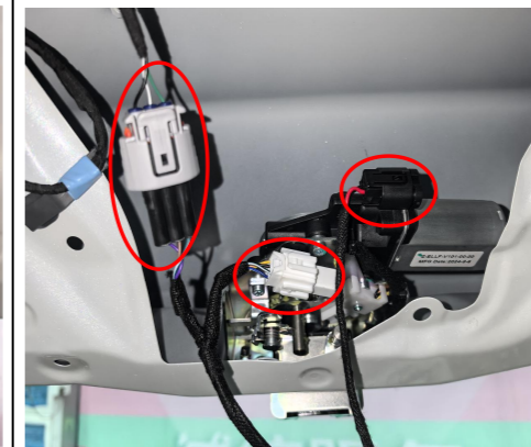
19. Connect the plugs of the lock signal harness to the plugs of the power latch.
