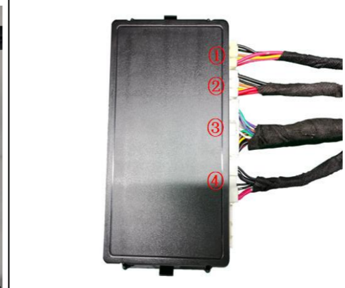
36. Insert the left and right strut wiring harnesses ①②, lock signal harness ③, and power harness ④ into the ECU in sequence.
