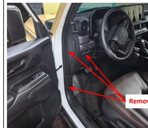
1. Remove the indicated front left side trim panels.
