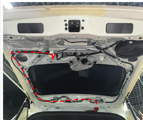
16. Route the strut wiring harness along with the original wiring harness.
