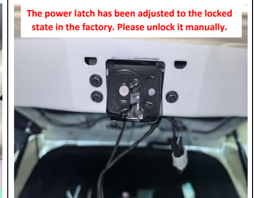
20. Install the power latch.
