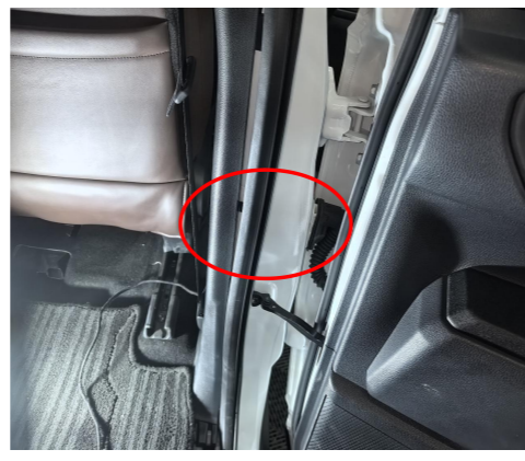
29. Find out the B-pillar plugs at the rear right B-pillar.
