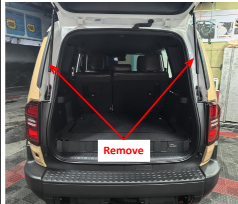
6. Remove the original gas struts.
