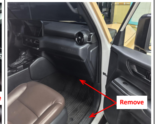
2. Remove the indicated front right side door panel and the fuse box trim panel.
