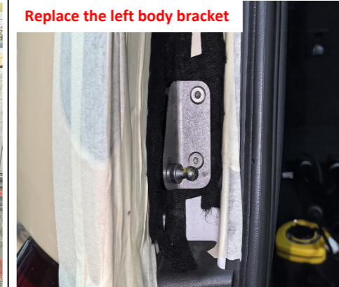
7. Replace the left body bracket.
