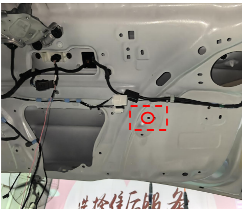
34. Secure the ECU bracket at the indicated position.
