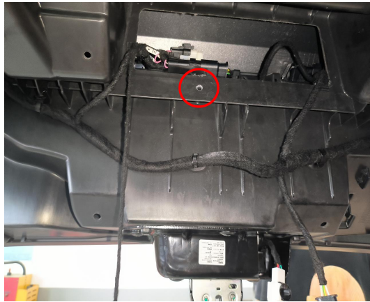
27. Drill a hole at the indicated position with a \phi 6 mm drill bit.
