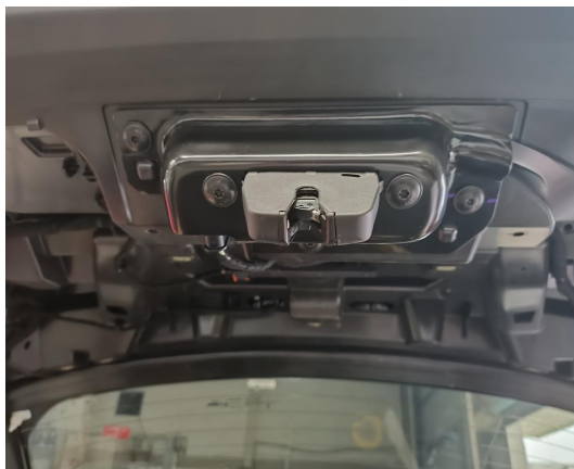
13. Remove the original latch.
