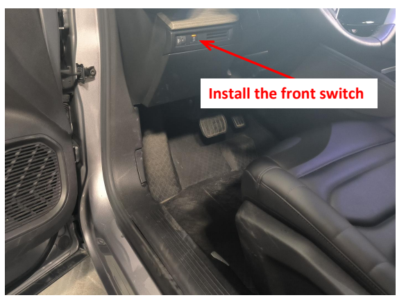
21. Remove the blank button from the switch panel for installing the front switch.
