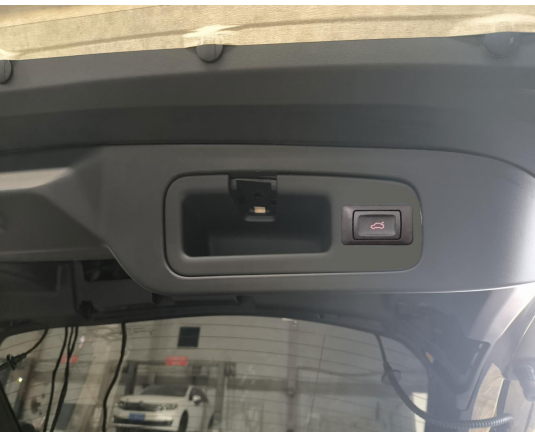
33. Install the added tailgate switch and reinstall all the trim panels.
