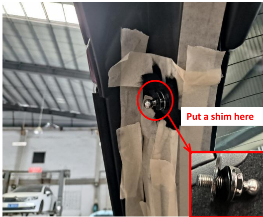
9. Replace the ball studs on both sides of the tailgate (pay attention to put a shim under the ball stud).
