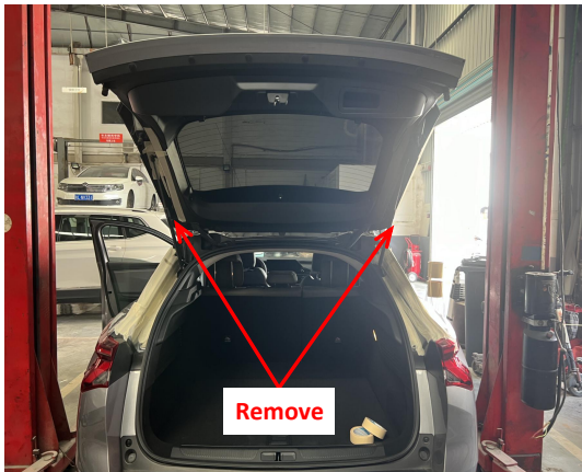
6. Remove the original gas struts.
