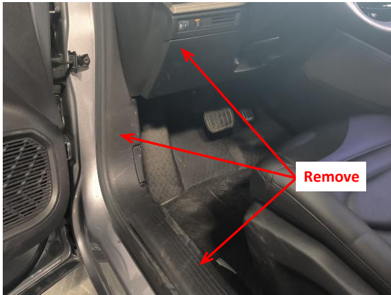
1. Remove the indicated driver's side trim panels.
