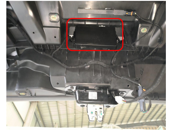
30. Fit the ECU into the bracket and tie the wiring harnesses to the original wiring harness.
