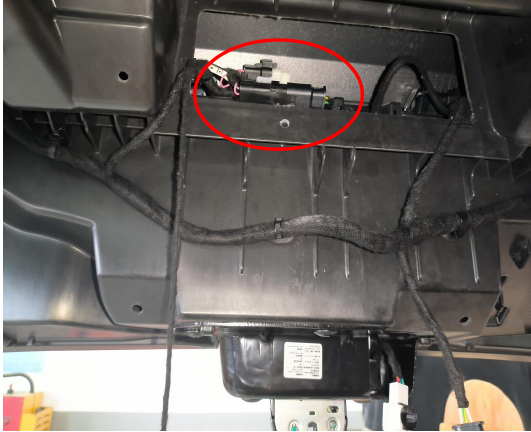
17. Connect the plugs of the lock signal harness to the plugs of original tailgate switch.
