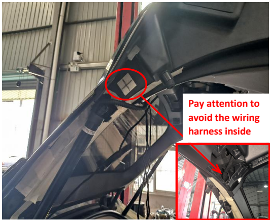
11. Drill a hole at the indicated position with a Ø21 drill bit to allow strut wiring harness to pass through.
