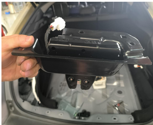
14. Fit the power latch into the metal casing of the original latch.
