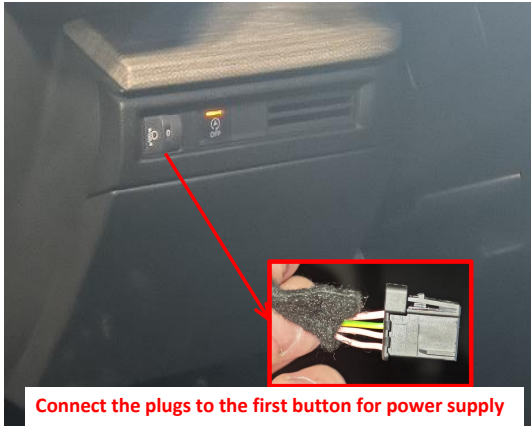
22. Connect the plugs of front switch to the first button.
