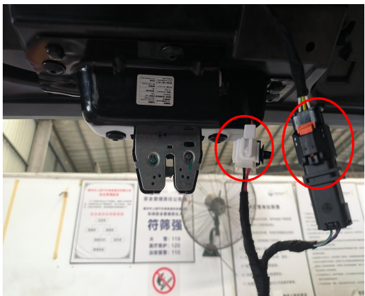
16. Connect the plugs of the lock signal harness to the plugs of the power latch.
