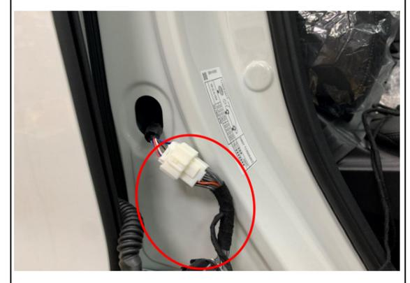
21. Connect the power harness to the indicated plugs at B-pillar.
