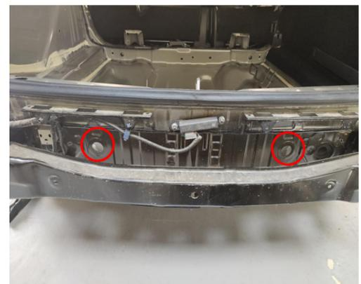
8. Thread the wiring harnesses through the holes of the bumper.
