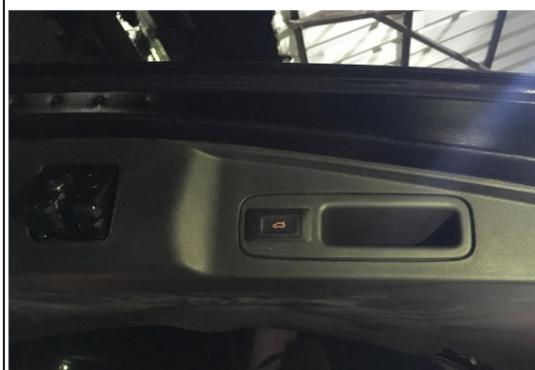
30. Install all the trim panels back and install the added tailgate switch.
