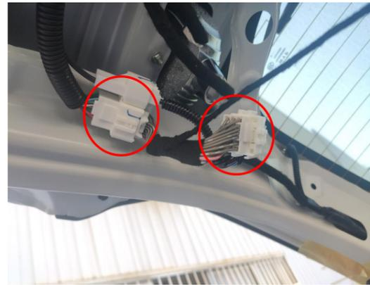
18. Connect the plugs of the lock signal harness to the plugs of the tailgate handle switch.
