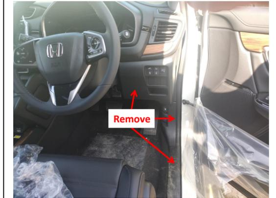
1. Remove the indicated front right side trim panels and door sill panel.
