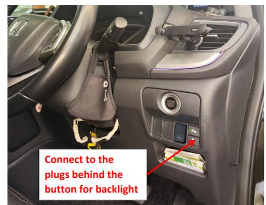
23. Connect the power harness to the plugs of the front switch behind the panel.
