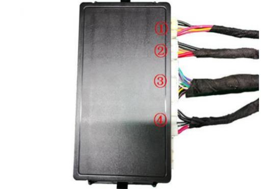
28. Insert the strut wiring harnesses ①②, lock signal harness ③, and power harness ④ into the ECU in sequence and mount the ECU onto its bracket.
