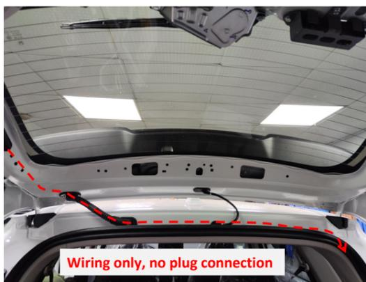
Wiring only, no plug connection
