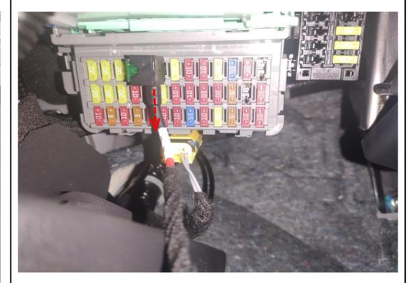
26. Move the original fuse from the fuse box to the fuse tap and then plug the fuse tap into the fuse box with wire
