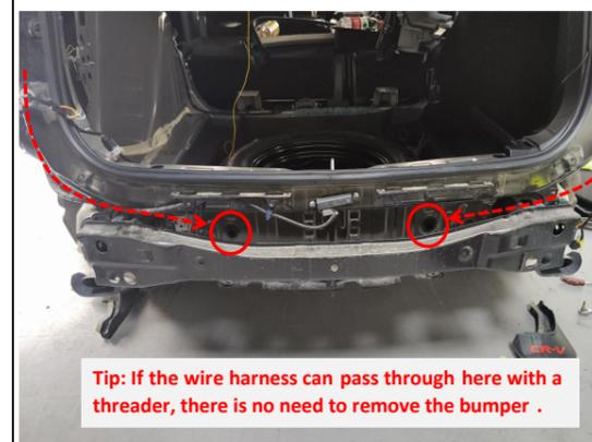
Tip: If the wire harness can pass through here with a threader, there is no need to remove the bumper.
