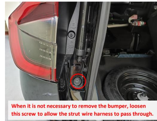
When it is not necessary to remove the bumper, loosen this screw to allow the strut wire harness to pass through.
