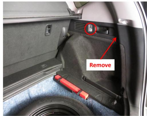
3. Take out the trunk floor mat and remove the trim panel on the right side of the trunk.
