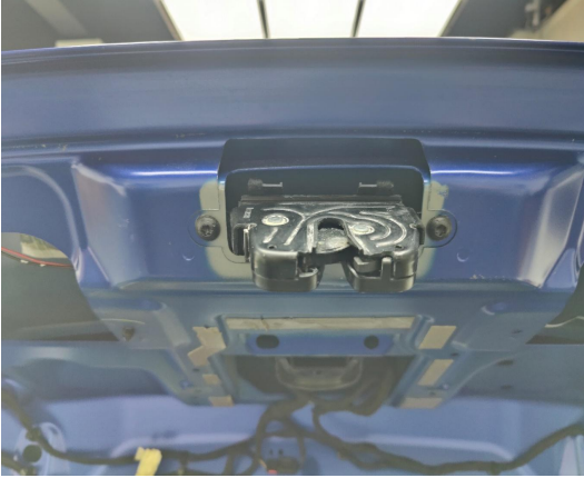
4. Remove the original latch and keep the two screws.
