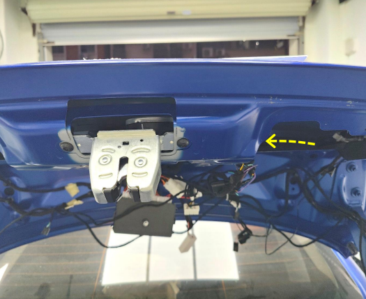
6. Install the power latch (put it in from the indicated hole and make sure the latch is locked).
