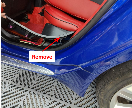
3. Remove the rear left door sill panel.
