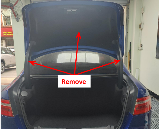
1. Remove the indicated trim panels from the tailgate and hinges.
