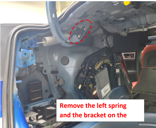
9. Remove the left spring and the bracket on the left hinge.
