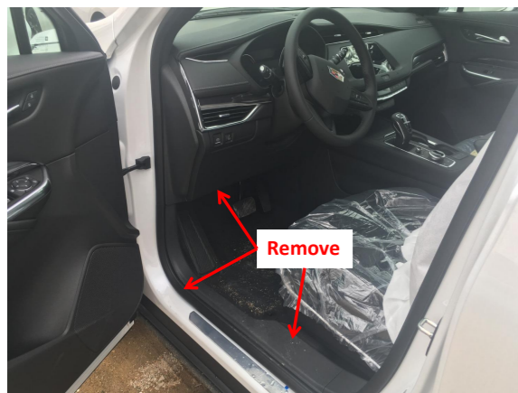
2. Remove the front left side trim panel, door sill panel and storage box.
