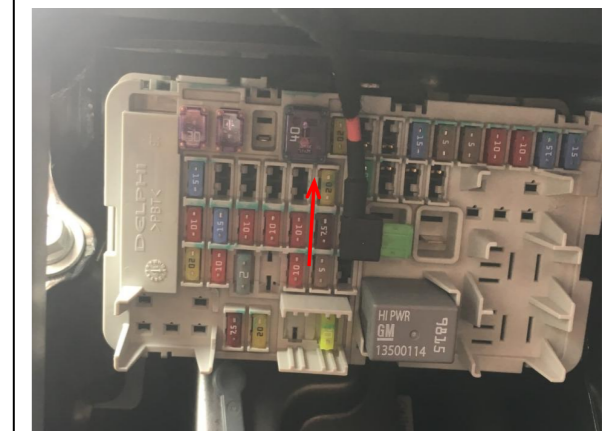
26. Plug the fuse tap into the fuse box and pay attention to the direction.
