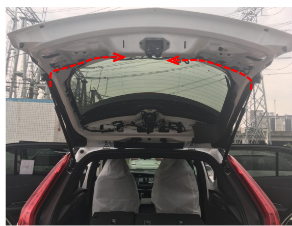
17. Thread the strut wiring harnesses into the tailgate.
