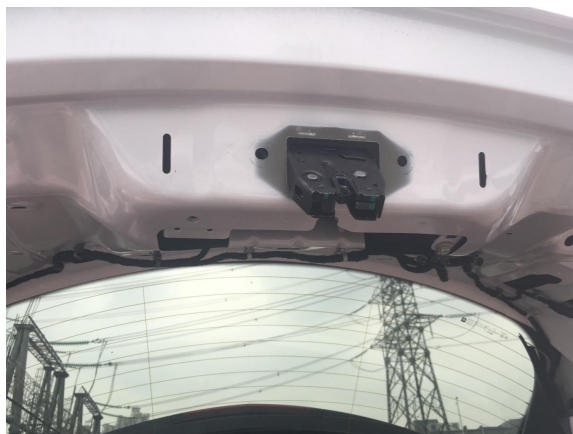
7. Remove the original latch.
