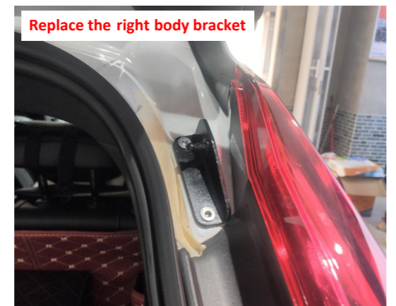
13. Replace the bracket on the right side of the car body.
