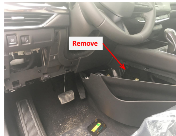
3. Remove the trim panel on the right side of the driver's seat.
