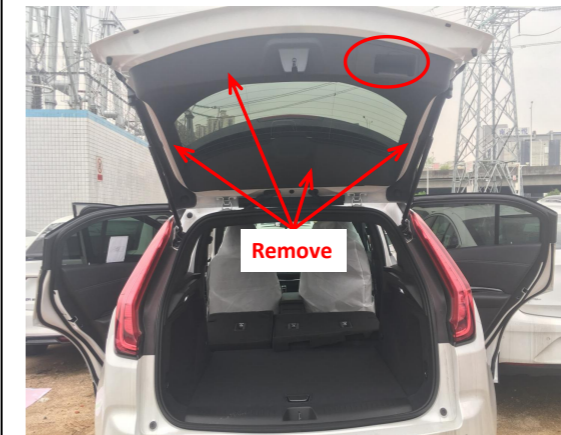
5. Remove the tailgate trim panels.
