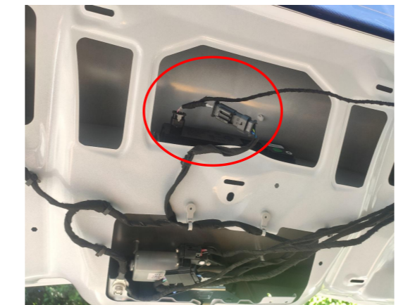
9. Connect the lock signal harness to the plugs of the original tailgate switch.
