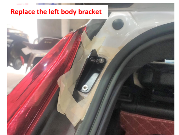
12. Replace the bracket on the left side of the car body.
