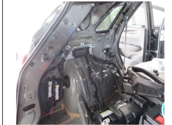
6. Remove the trim panel on the left side of the trunk to allow wiring harnesses to pass through.
