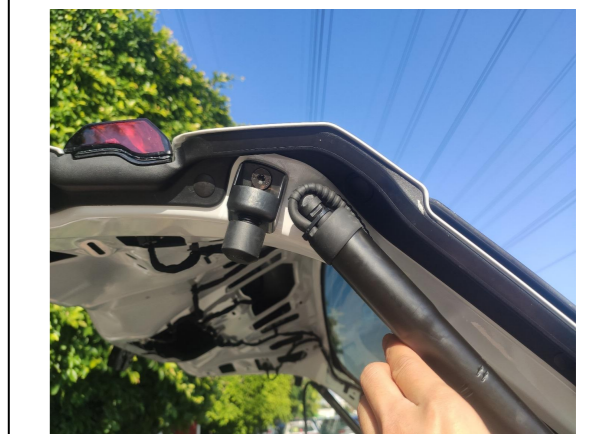
16. Tie the rubber tube with the strut as shown above and plug the hole securely; both sides are the same.
