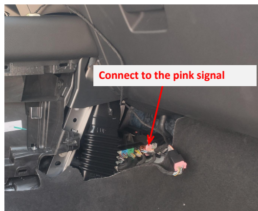
22. Connect the power harness to the indicated pink signal plug and its socket.
