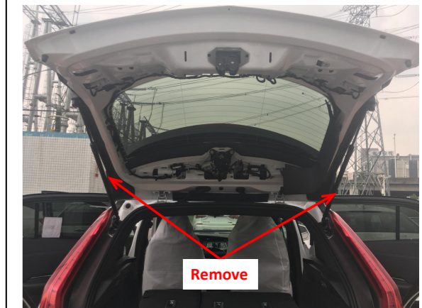
11. Remove the original gas struts.
