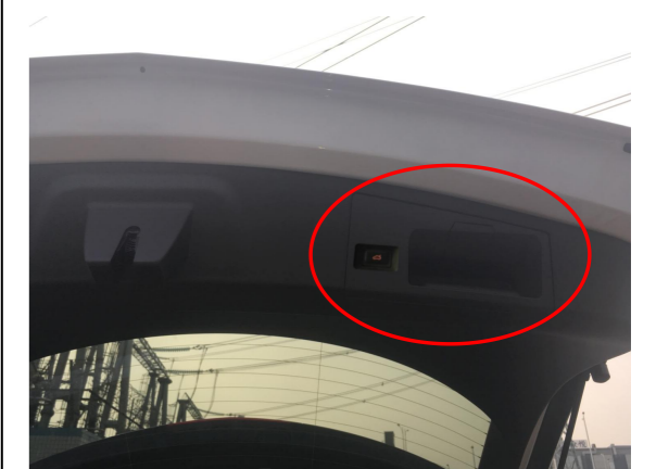
31. Reinstall all trim panels and install the added tailgate switch (replace the original tailgate handle).
