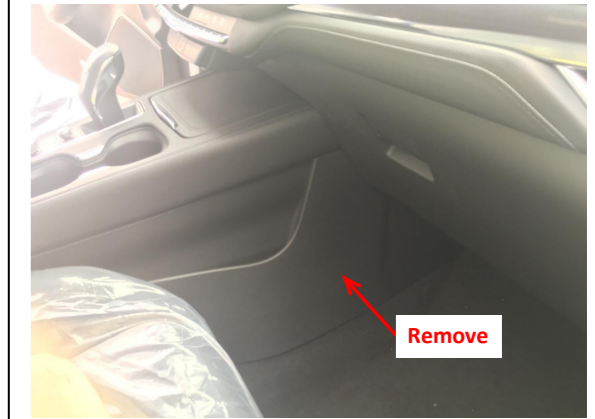
1. Remove the trim panel on the left side of the front passenger seat.
