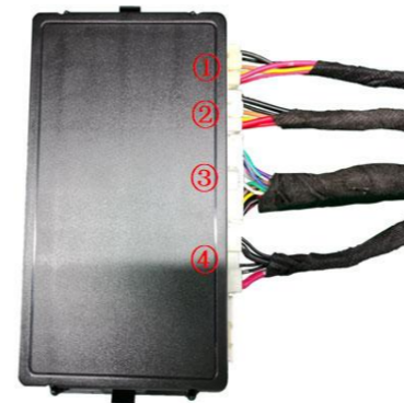
29. Insert the strut wiring harnesses ①②, lock signal harness ③, and power harness ④ into the ECU in sequence and then mount the ECU onto its bracket.
