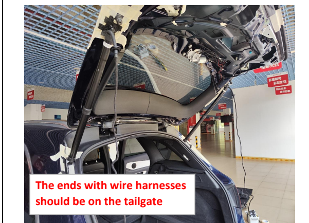
6. Install the electric struts, L on the left and R on the right (the first letter of the strut code).
