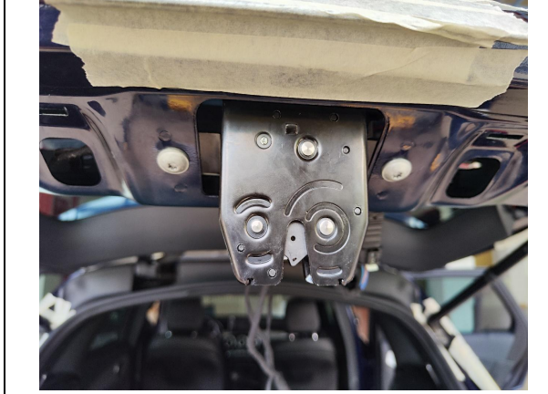
11. Remove the original latch and install our power latch.
