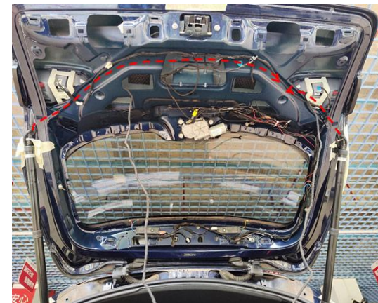
8. Route the left and right strut wiring harnesses to the right side of the tailgate.
