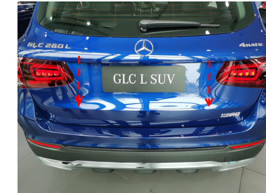
25. Press the added tailgate switch to open and close the tailgate once, the system completes initialization, and then test each function of the electric tailgate.
