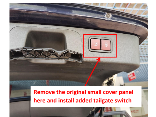
26. Reinstall all the trim panels and install the added tailgate switch.
