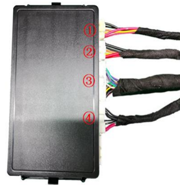
23. Insert the strut wiring harnesses ① ②, lock signal harness ③, and power harness ④ into the ECU in sequence.
