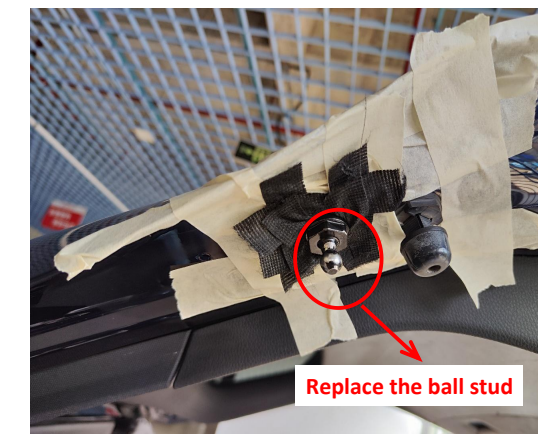
5. Replace the left and right ball studs with our reinforcing ball studs.
