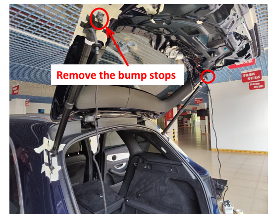
7. Thread the strut wiring harnesses through the holes for bump stops on the left and right sides of the tailgate.
