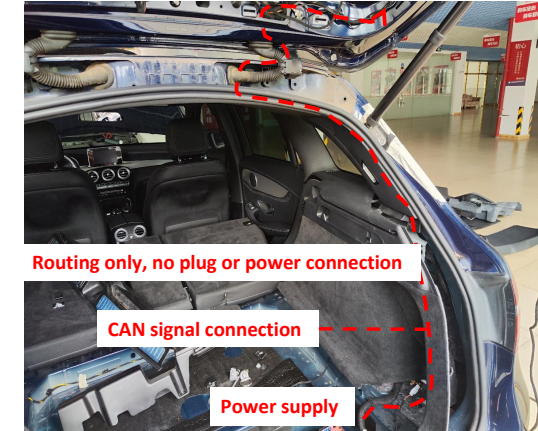
15. Route the power harness to the right side of the tailgate.
