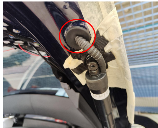
9. Plug the holes on the left and right sides of the tailgate.
