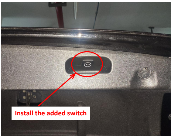
33. Install all trim panels back and install the added tailgate switch.
