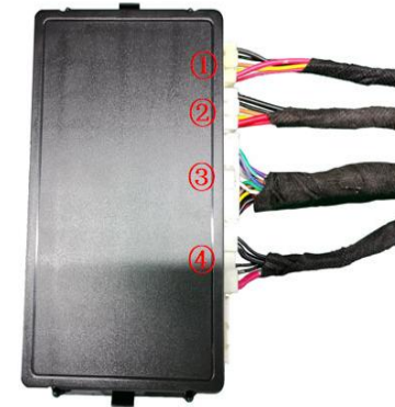
30. Insert the strut wiring harnesses ① ②, lock signal harness ③, and power harness ④ into the ECU in sequence.
