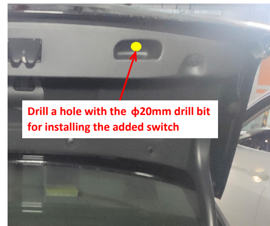
32. Drill a hole at the indicated position for the installing the added switch
