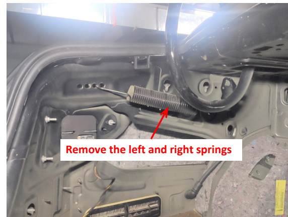
4. Remove the left and right springs from the trunk.
