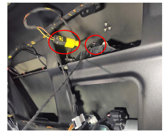
21. Connect the plugs of lock signal harness to the plugs of original tailgate switch and the added switch.
