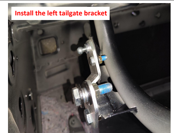
8. Install the tailgate bracket on the left hinge.
