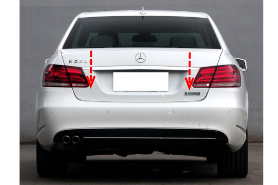
31. Manually close the tailgate until it touches the striker, then press the original tailgate switch button to open the tailgate. The system initialization is complete, and then test each function of the electric tailgate.
