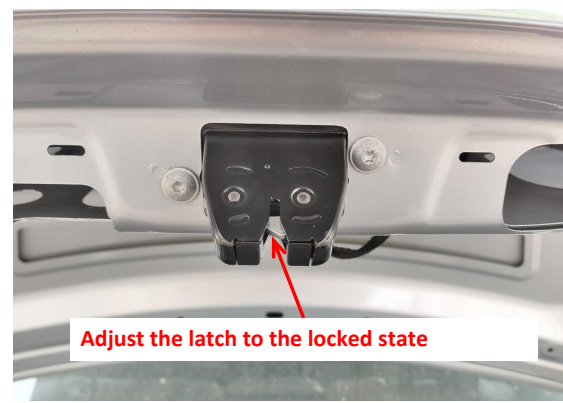
18. Install the lock actuator and secure it with original screws. Manually adjust the latch to the locked state to prevent accidental closing during the installation process.
