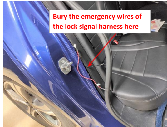
22. Route the emergency wires of the lock signal harness along the right hinge to the right side of rear seat (the emergency wires should be in place for emergency use).
