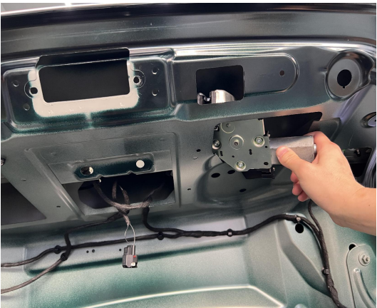
16. Put the power latch into the tailgate from the right side of the tailgate.
