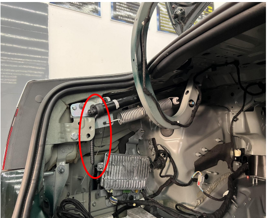
11. Install the electric struts with L on the left and R on the right (the first letter of the strut code).
