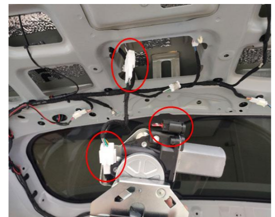
7. Connect the plugs of the lock signal harness to the power latch.
