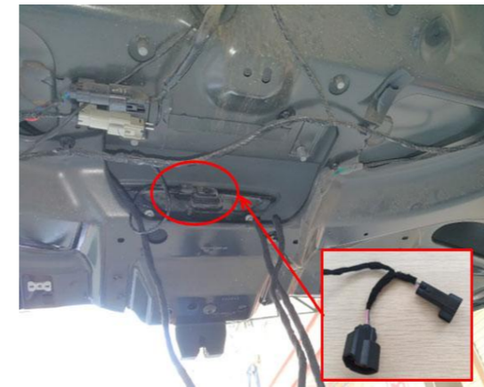
9. Connect the plugs of the lock signal harness to the plugs of the original tailgate switch and the added tailgate switch.
