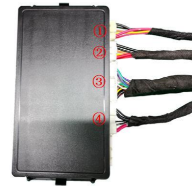
24. Insert the strut wiring harnesses ①②, lock signal harness ③, and power harness ④ into the ECU in sequence.
