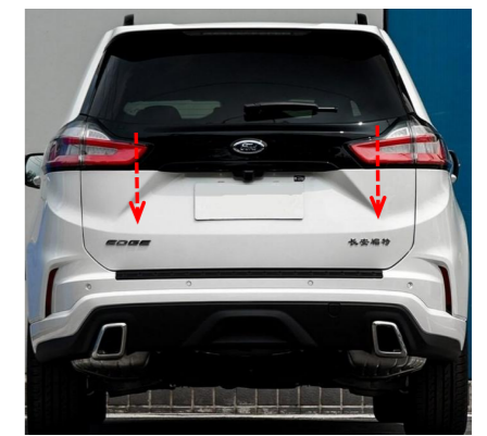
25. Press the added switch on the tailgate to open and close the tailgate once for initializing the system, and then test each function of the electric tailgate.
