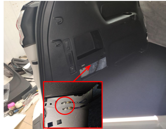
18. Ground at the left side of the trunk.
