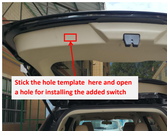
26. Stick the hole template to the indicated position and open a hole for installing the added tailgate switch.
