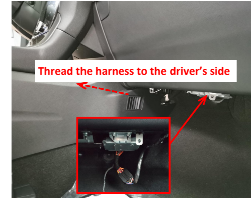
19-2. For 2020-2021 Edge Plus, connect the plugs of power harness to the CAN plugs under the storage box of the passenger seat and then thread the harness to the driver's side.
