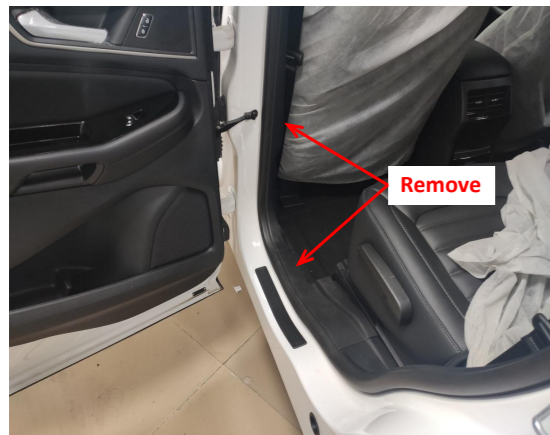
2. Remove the rear left side door sill panel and B-pillar trim panel.
