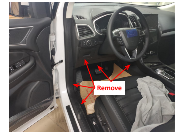
1. Remove the trim panels and door sill panel in the driver's area.
