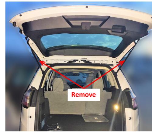
10. Remove the original gas struts.
