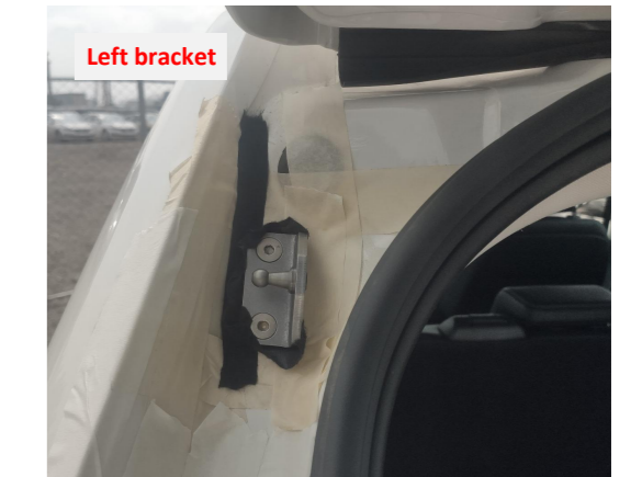
11. Replace the left bracket on the car body.
