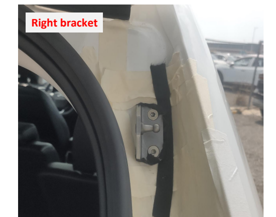
12. Replace the right bracket on the car body.
