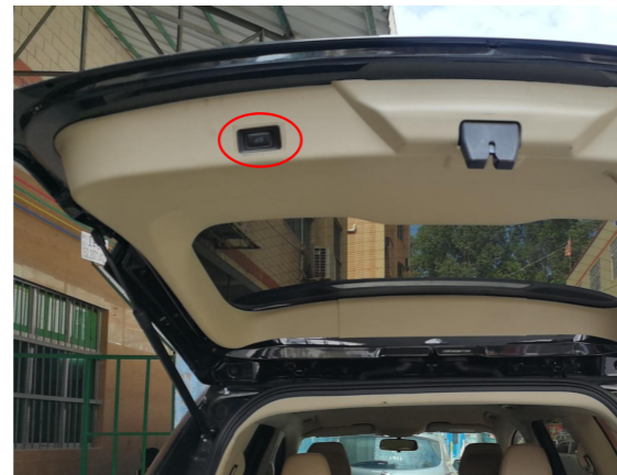
27. Reinstall all trim panels and install the added tailgate switch.
