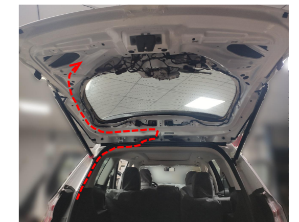
16. Route the power harness to the left side of the trunk.
