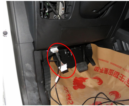
19. For models during 2015-2019, connect the plug of the power harness to the indicated OBD plug.
