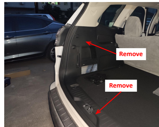
4. Remove the door sill panel and left side trim panel from the trunk.
