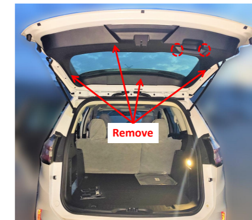
5. Remove the tailgate trim panels (there are screws inside the circles).
