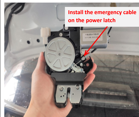
17. Install the emergency cable on the power latch (inside fastener).
