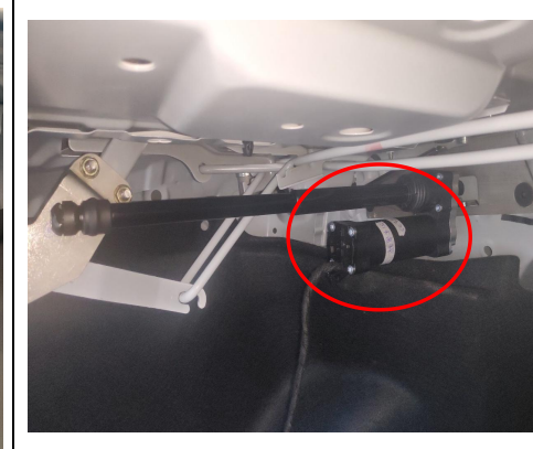
13. Install the electric struts, L on the left and R on the right (the first letter of the strut code), making sure the ends with wiring harnesses are on the car body.
