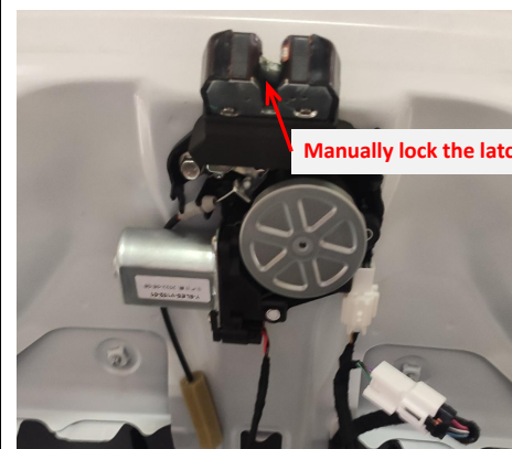
18. Install our power latch and manually adjust the latch to the locked state.
