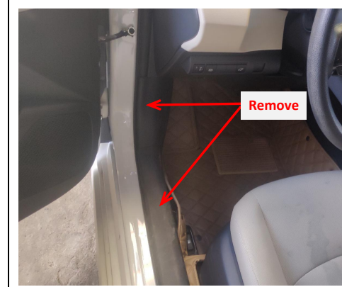
1. Remove the front left door sill panels.
