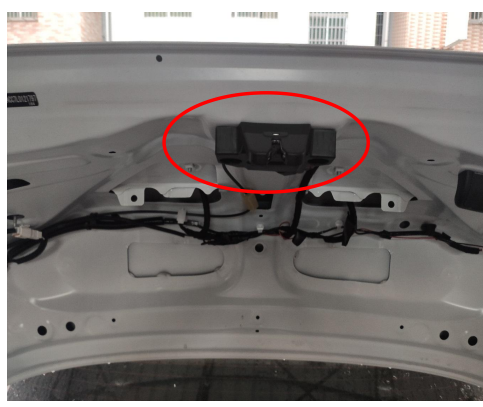
16. Remove the original latch and the emergency lock cable.
