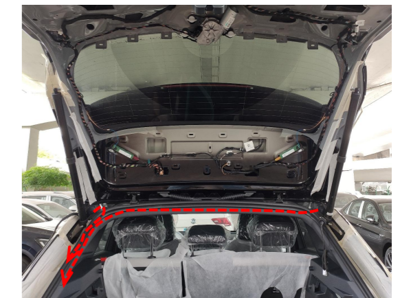
11. Route the strut wiring harnesses to the left side of the trunk.
