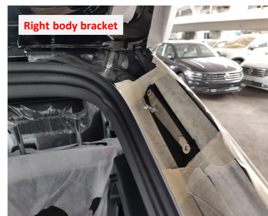
8. Replace the right body bracket.
