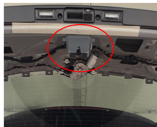
13. Remove the original latch.
