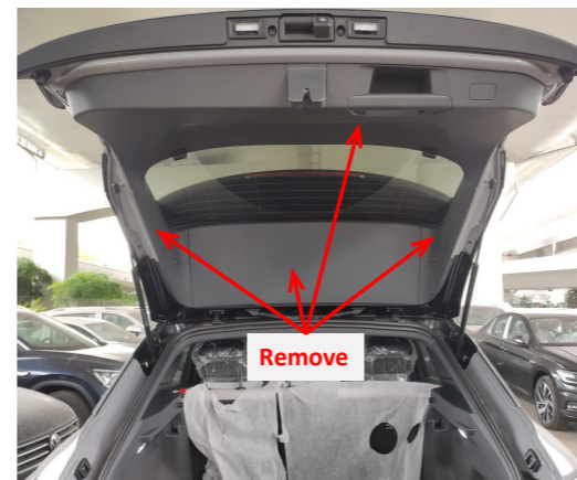
4. Remove the tailgate trim panels.
