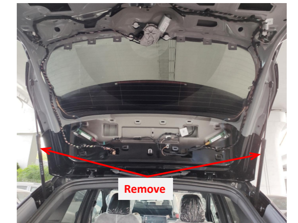
6. Remove the original gas struts.
