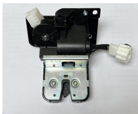
14. Remove the plastic housing from the power latch and cut off the cable tie.
