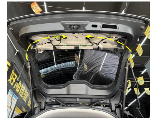
6. Route the strut wiring harnesses as indicated.
