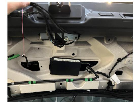
23. Fit the ECU onto its bracket.
