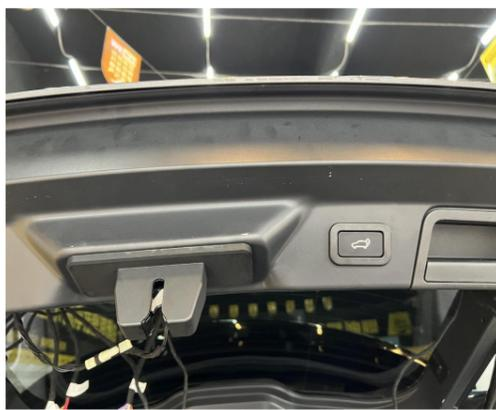
27. Install the added tailgate switch and reinstall the trim panels.
