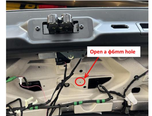
21. Open a  $\phi 6\text{mm}$  hole at the indicated position.
