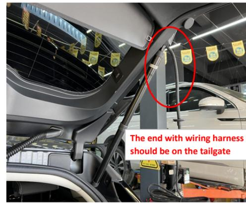
4. Install the electric struts, L on the left and R on the right (the first letter of the strut code).
