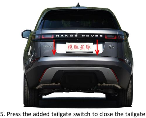
25. Press the added tailgate switch to close the tailgate once, the system completes initialization, and then test each function of the electric tailgate.
