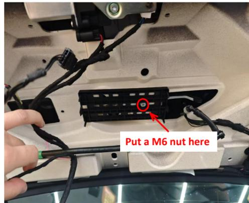
22. Install the ECU bracket with the hexalobular socket screw.
