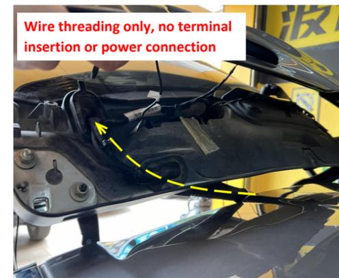
15. Thread the power harness through the indicated position under the spoiler.
