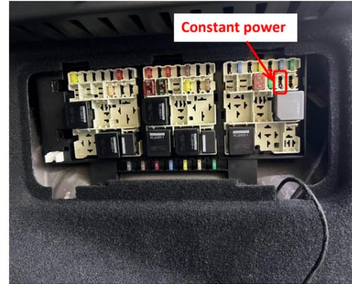
19. The fuse box is located at the right side of the trunk and the fuse slot for power supply is indicated.
