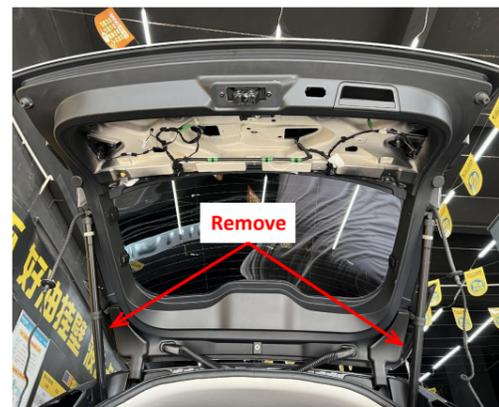
13. Remove the hinge trim panels on both sides.
