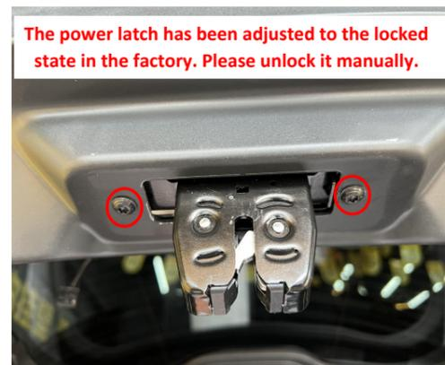
9. Install the power latch and the plastic casing.
