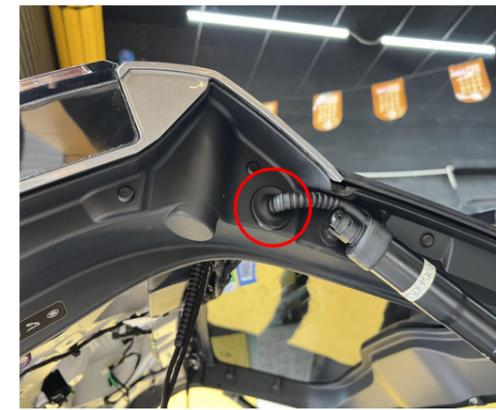
5. Thread the strut wiring harness through the indicated hole into the tailgate, the same on both sides.
