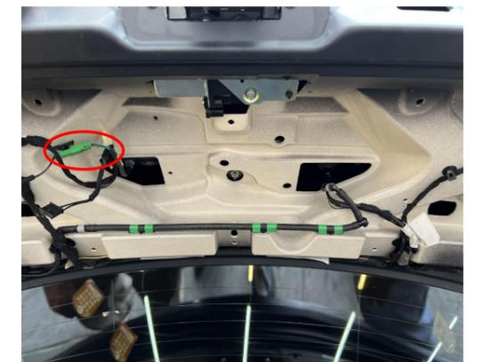
11. Connect the plugs of the lock signal harness to the plugs of the original tailgate switch.
