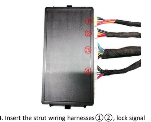
24. Insert the strut wiring harnesses ① ②, lock signal harness ③, and power harness ④ into the ECU in sequence.
