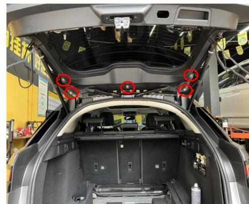
14. Remove the indicated 5 screws and remove the spoiler.
