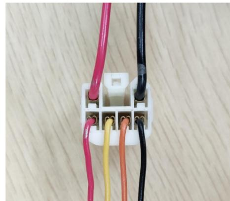
7. Insert the strut wiring harness terminals into the connector (on the ECU) according to the diagram.
