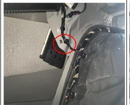
32. Drill a hole at the indicated position for installing the added tailgate switch.
