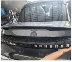
16. Remove the screws from the taillights on both sides | 17. Remove the taillight and find out the plug of original tailgate switch.
