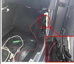
28. Connect to the CAN signal plugs at the right side of the front passenger seat.
