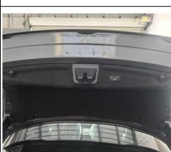
1. Manually adjust the latch to the locked
