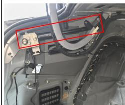
13. Install the electric struts, L on the left and R on the right (the first letter of the strut code).
