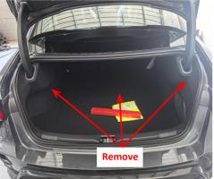
I. Remove the trunk floor mat and the trim panels on both sides.
