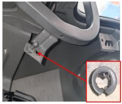
3. Remove the iron fasteners on both sides used for hanging springs.
