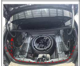
15. Route the strut wiring harnesses along with original wiring harness.
