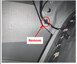
30. Remove the indicated cable tie on the left side of the tailgate.
