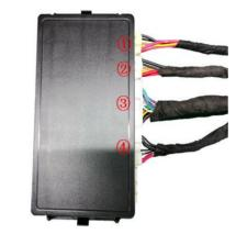
29. Insert the left and right strut wiring harnesses (1)lock signal harness 3, and power harness 4 into the ECU in sequence.
