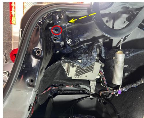
7. Thread the M10 nut with a handle to the indicated position to install the left body bracket.
