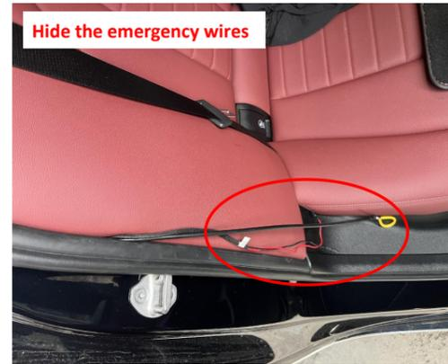
20. Hide the two emergency wires of the power latch under the trim panel of the rear right seat.
