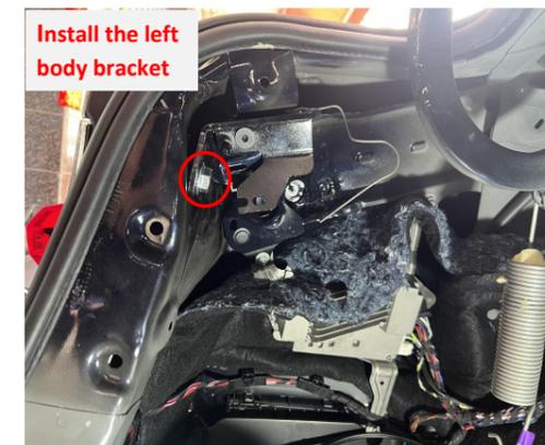
10. Screw the M12 screw into the nut to finish the installation of the left body bracket.
