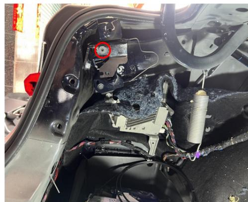
8. Screw the countersunk screw into the nut.
