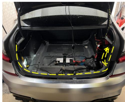
13. Route the strut wiring harnesses to the right side of the trunk along with original wiring harness.
