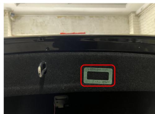
33. Stick the provided hole template to the indicated position and open a hole for the added tailgate switch.
