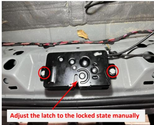
17. Install the power latch and adjust the latch to the locked state manually.
