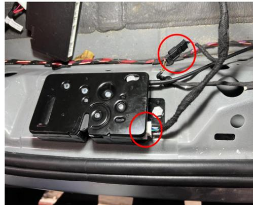
18. Connect the plugs of the lock signal harness with the power latch.
