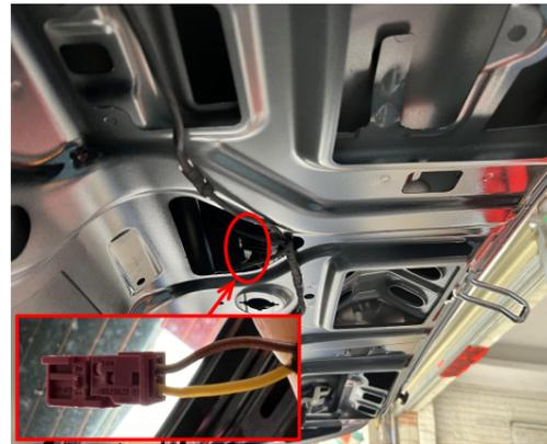
19. Connect the plugs of the lock signal harness with the original tailgate switch.
