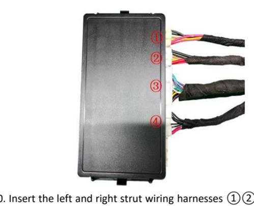
30. Insert the left and right strut wiring harnesses ①②, lock signal harness ③, and power harness ④ into the ECU in sequence.
