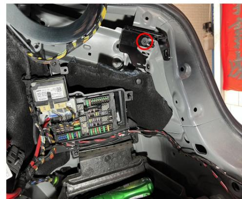
4. Screw a countersunk screw into the indicated threaded hole.
