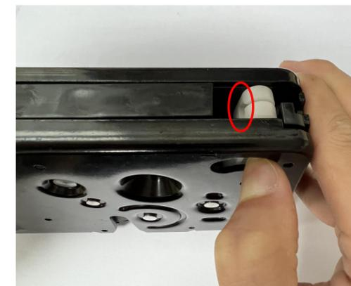
15. Install the emergency cable and unfasten the unlock arm.
