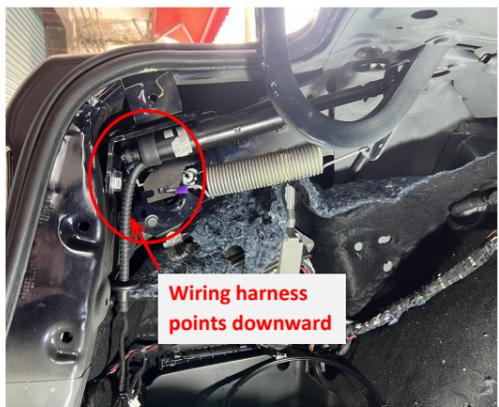
12. Install the electric struts, L on the left, R on the right (the first letter of the strut number); the same on both sides.
