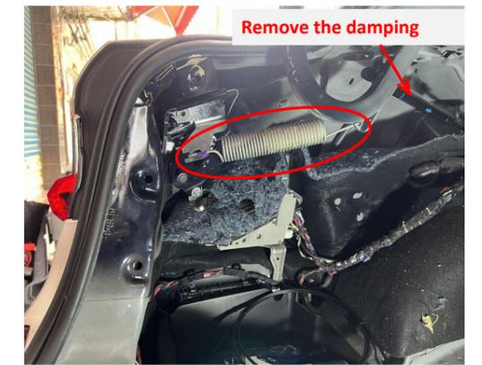
11. Hang the original springs at the left and right body brackets, then remove the damping rod on the left side.
