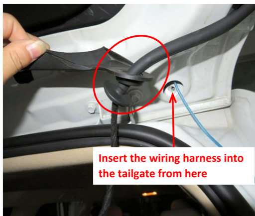
12. Thread the strut wiring harness through the indicated hole and then plug the hole.
