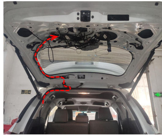
18. Route the power harness to tailgate.
