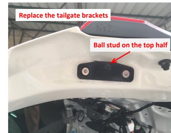
8. Replace the left and right tailgate brackets with the ball studs on the top half.
