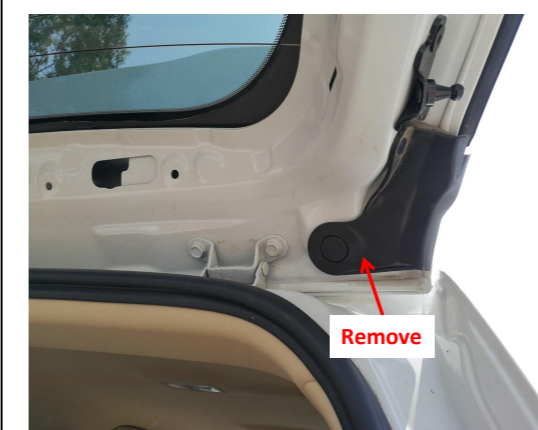
10. Remove the left and right tailgate rubber pads.
