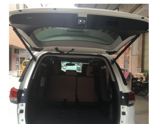
30. Reinstall all the trim panels and install the added tailgate switch.
