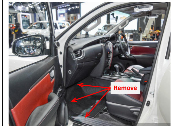
1. Remove the indicated trim panels and door sill panel to find out the fuse box.
