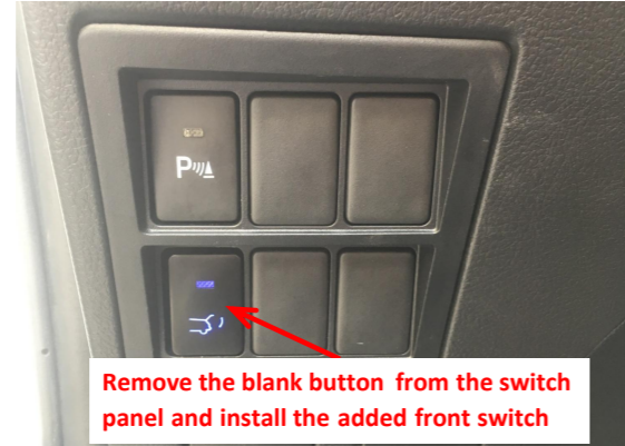
23. Remove the blank button from the switch panel, install the front switch, and connect to the plugs of the switch beside it for backlight.
