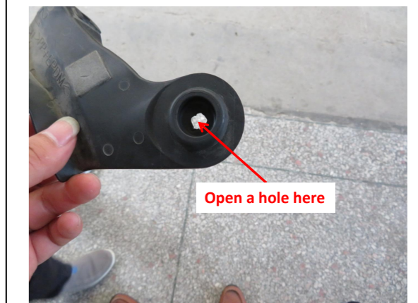
11. Open a hole at the indicated position of the rubber pads to allow the strut wiring harnesses to pass through.
