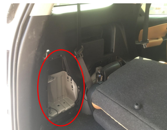
3. Remove the trim panel on the left side of the trunk to allow wiring harnesses to pass through.
