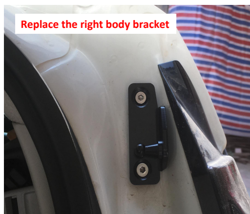
7. Replace the right body bracket.
