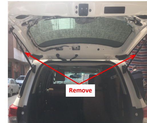
5. Remove the original gas struts.
