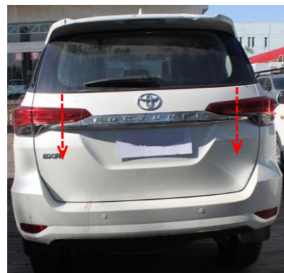
28. Press the added tailgate switch to open and close the tailgate once, the system completes initialization, and then test the functions of the electric tailgate.
