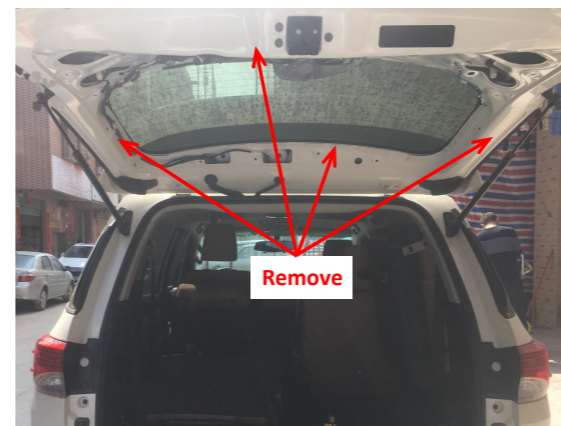
4. Remove the tailgate trim panels.
