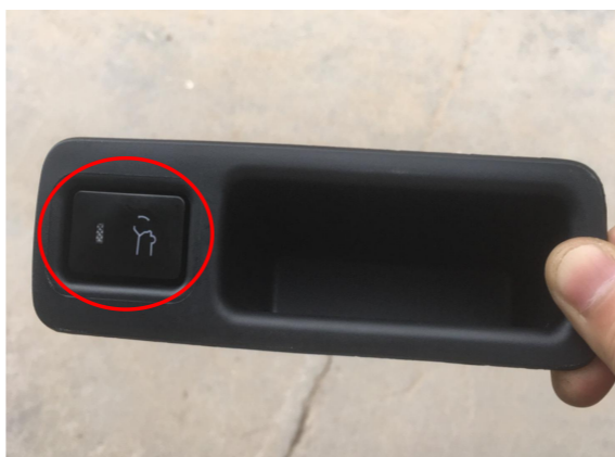
29. Install the added tailgate switch button on the tailgate handle.
