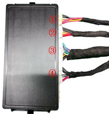
27. Insert the strut wiring harnesses ①②, lock signal harness ③, and power harness ④ into the ECU in sequence, and mount the ECU on its bracket.
