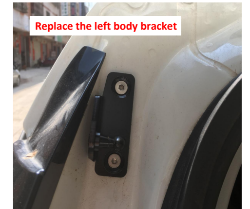
6. Replace the left body bracket.
