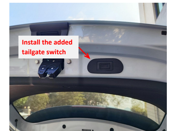
31. Reinstall all trim panels and install the added tailgate switch.
