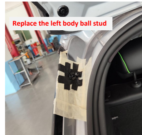
8. Replace the left body ball stud with provided one.
