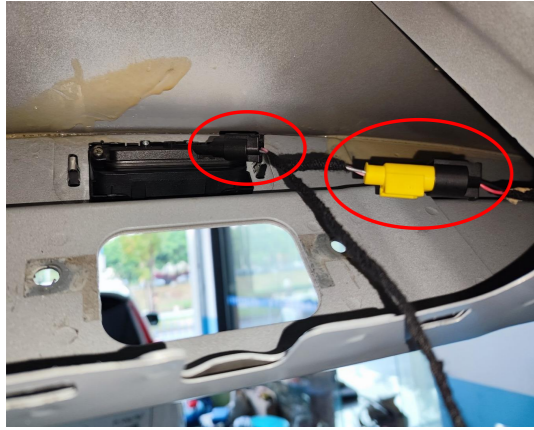
17. Connect the plugs of lock signal harness to the original tailgate switch behind the power latch.
