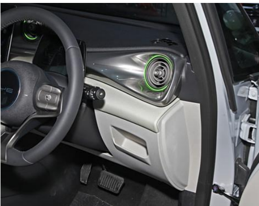
(Optional) Drill a hole with a \phi 21\text{mm} drill bit at an appropriate position and install the added front switch.
