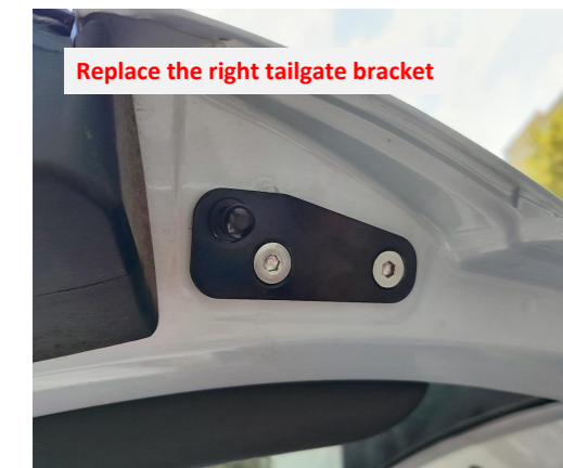
7. Replace the right tailgate bracket with provided one.
