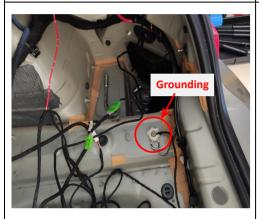
27. Ground at the indicated position on the right side of the trunk. The grounding wire must be installed as shown in the diagram.
