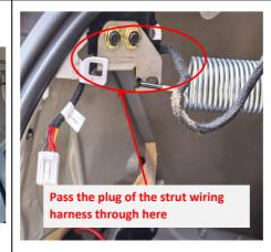
18. Pass the plug of the strut wiring harness through the indicated position.
