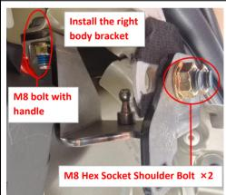
9. Secure the bracket on the original holes. Install the M8 bolt first, then install the M10 bolts.
