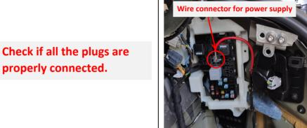
31. Connect to the fuse box on the right side of the trunk for power supply.
