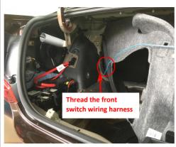
23. Thread the front switch wiring harness(the green plugs) to the driver's area.
