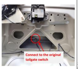
21. Connect the plugs of the lock signal harness to the plugs of original tailgate switch.
