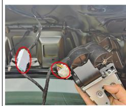
19. Remove the original latch and install our power latch. 20. Connect the plugs of the lock signal harness to the plugs of power latch.
