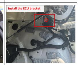
32. Secure the ECU bracket at the indicated position.
