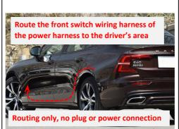
24. Route the front switch wiring harness of the power arness to the driver's area.
