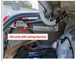
14. Install the electric struts, L on the left and R on the right (the first letter of the strut code). The end with wiring harness should be on the car body.
