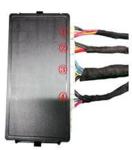
lock signal harness (3), and power harness (4) into the ECU in sequence.
