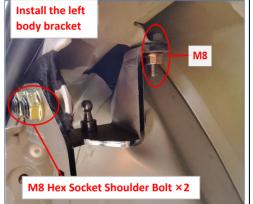
7. Secure the bracket on the original holes. Install the M8 8. Install the right body bracket on the right side of the bolt first, then install the M10 bolts.
