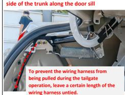
Route the left strut wiring harness to the right
