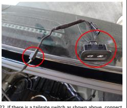
22. If there is a tailgate switch as shown above, connect it to the plug of lock signal harness. If there is no such tailgate switch, connect the provided tailgate switch to the plug of lock signal harness.
