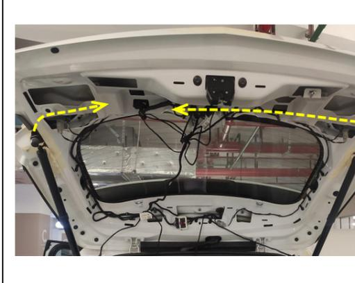
10. Route the strut wiring harnesses and plug the holes with hole plugs.
