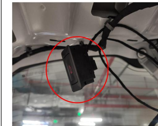
15. Connect the lock signal harness to the added tailgate switch.
