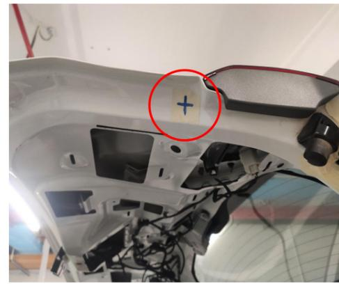
9. Drill a hole at the indicated position with a  $\phi 21$ mm drill bit on both sides of the tailgate.
