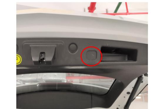
28. Stick the hole template to the reserved position of tailgate switch and open a hole to install the added tailgate switch.
