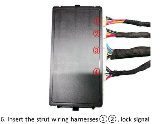
26. Insert the strut wiring harnesses ① ②, lock signal harness ③, and power harness ④ into the ECU in sequence.
