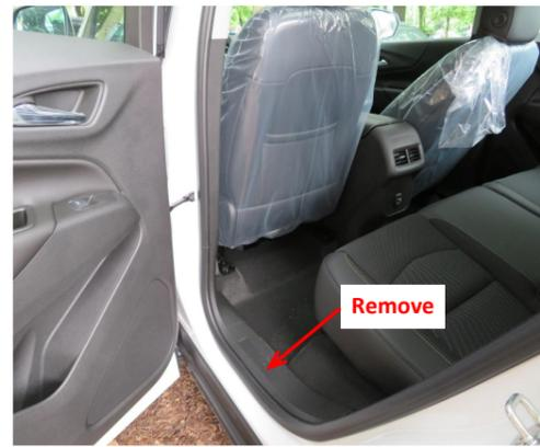
3. Remove the rear left side door sill panel.
