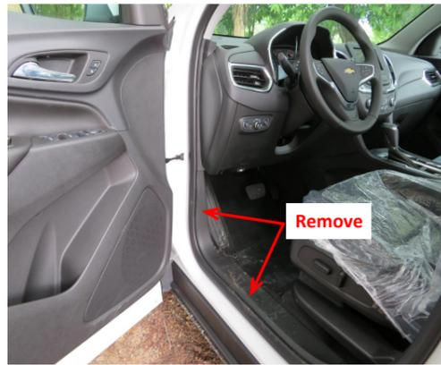
2. Remove the front left side trim panel and door sill panel.
