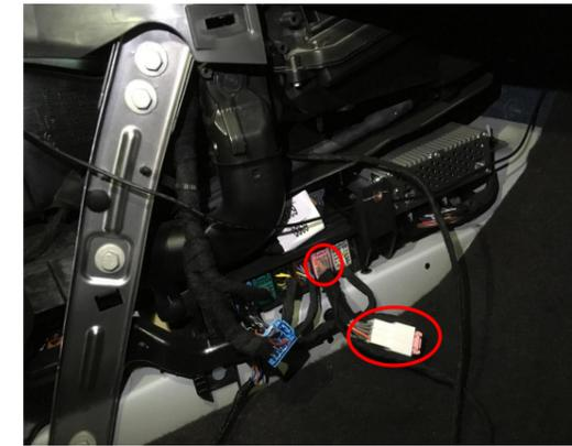
20. Connect to the indicated pink plug and its socket at the left side of the passenger seat for signal connection.
