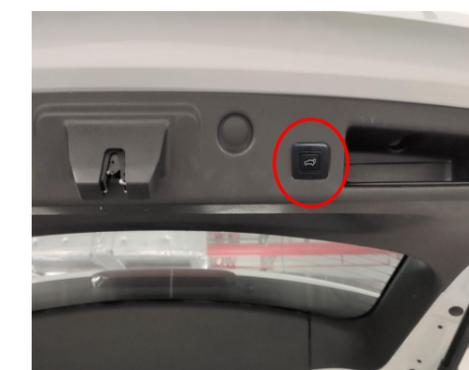
29. Reinstall all the trim panels and install the added tailgate switch.
