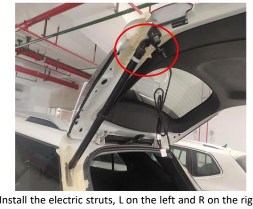
8. Install the electric struts, L on the left and R on the right (the first letter of the strut code), making sure the ends with wiring harnesses are on the tailgate.
