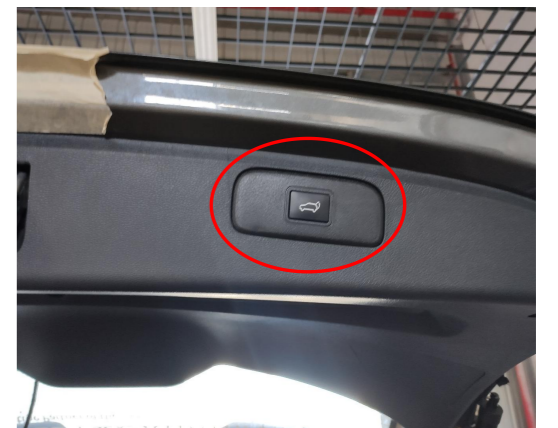
31. Install all trim panels back and fit the added tailgate switch in (remove the original small cover).
