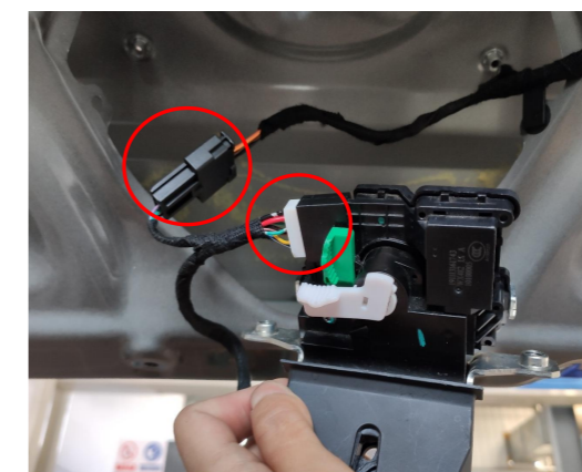
15. Connect the plugs of the lock signal harness to the power latch.
