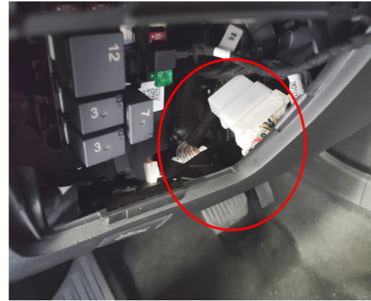
24. Connect to the OBD plug at the driver's position.
