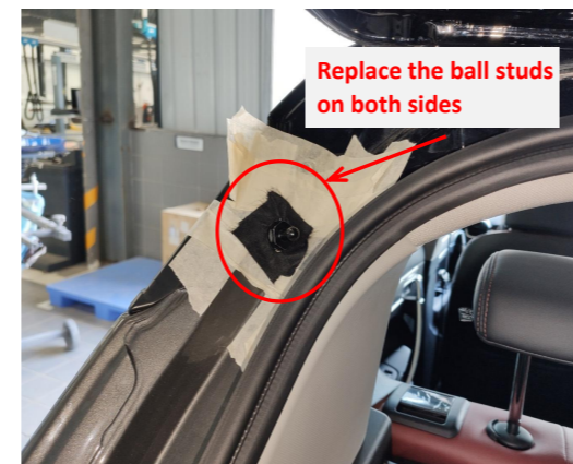
9. Replace the ball the studs on both sides.
