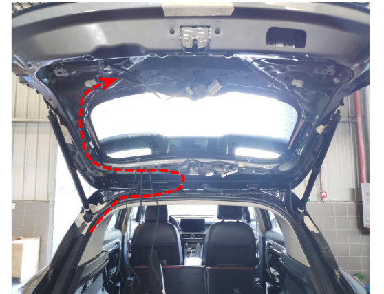
21. Thread power harness to the tailgate.
