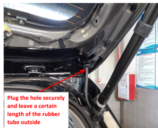
13. Leave a certain length of rubber tube outside to prevent it from being pulled during the movement of tailgate.
