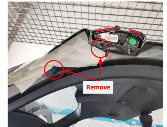
6. Remove the indicated ball stud and the nut on the tailgate lamp.
