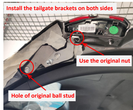
7. Install the tailgate brackets on both sides.
