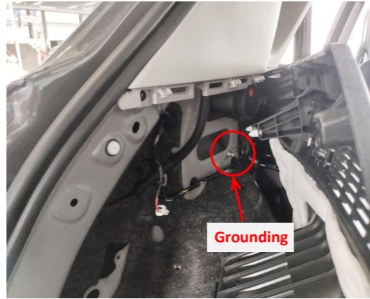
23. Ground at the indicated position on the left side of the trunk.
