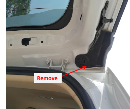
5. Remove the indicated rubber pad to allow the strut wiring harness to pass through. Both sides are the same.
