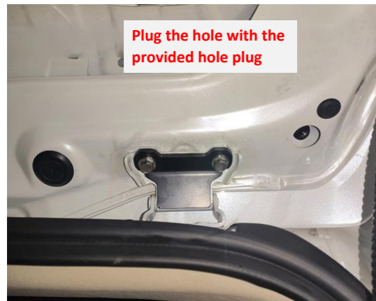
7. Plug the holes on both sides with the provided hole plugs.
