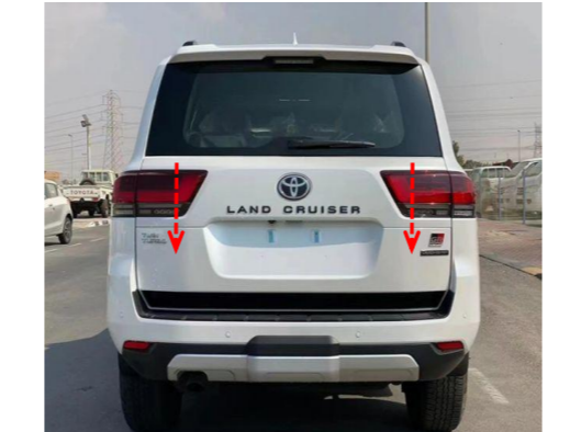
29. Press the tailgate switch buttons to open and close the tailgate once, the system completes initialization, then test each function of the electric tailgate.
