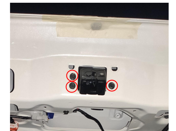
16. Remove the original latch and install the power latch.
