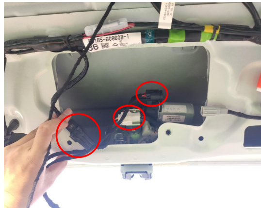
17. Connect the plugs of lock signal harness to the power latch.
