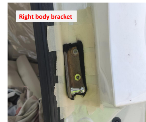
10. Install the bracket on the right side of the vehicle body.
