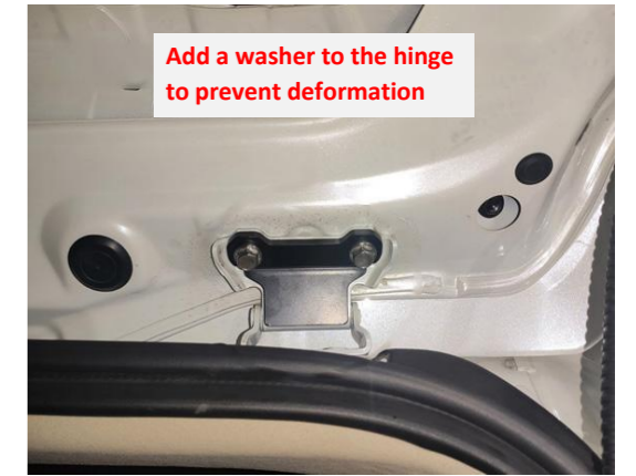
6. Add a washer to the hinges on both sides of the tailgate and secure them with provided screws.
