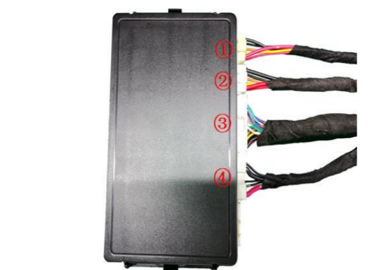
28. Insert the left and right strut wiring harnesses ①②, lock signal harness ③, and power harness ④ into the ECU in sequence.
