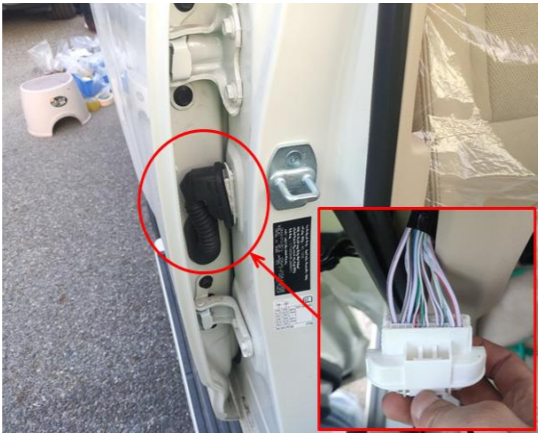
23. Connect the B-pillar signal at the rear right side B-pillar.
