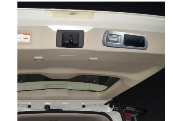
30. Reinstall all the trim panels and install the added tailgate switch.
