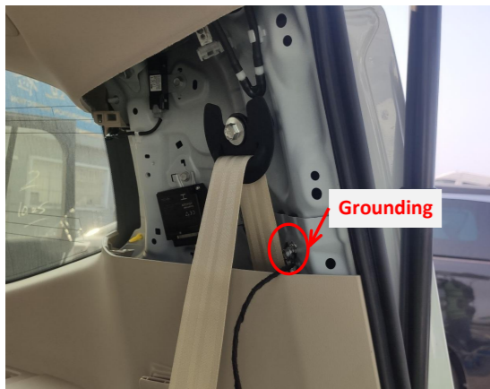
22. Ground at the right side of trunk.
