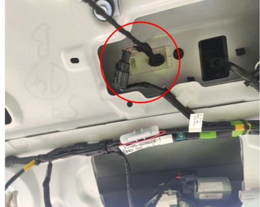
18. Connect the tailgate switch signal: connect the plugs of the lock signal harness to the original tailgate switch.
