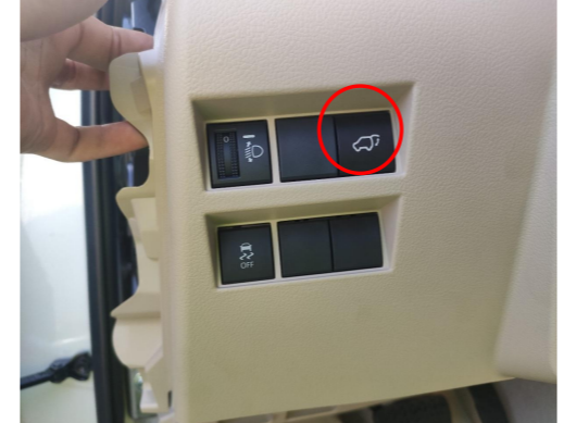
24. Remove the blank button from the switch panel, install the front switch and connect the plugs with the switch beside it to make the button light up.
