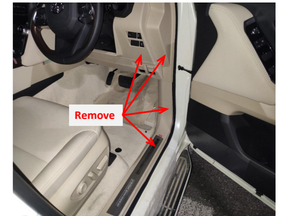
1. Remove the front right side trim panel, door sill panel and switch panel.
