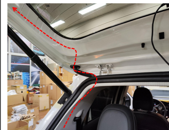
15. Thread the power harness to the tailgate.
