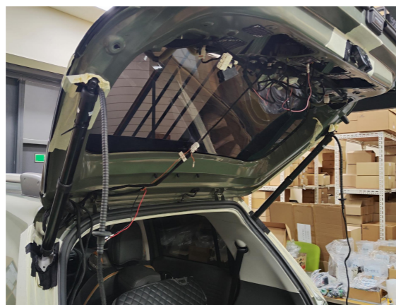
8. Install the electric struts, L on the left and R on the right (the first letter of the strut code). Pay attention to the
