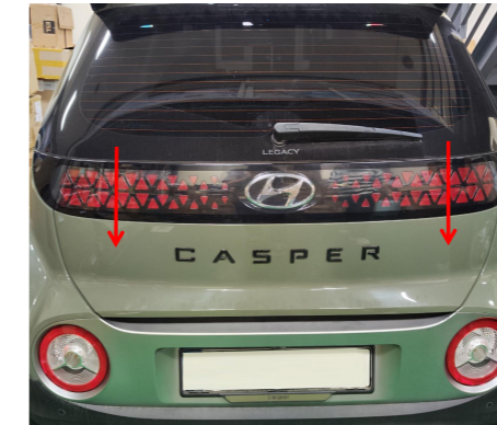
25. Press the added tailgate switch to close the tailgate once, the system completes initialization, and then test each function of the electric tailgate.
