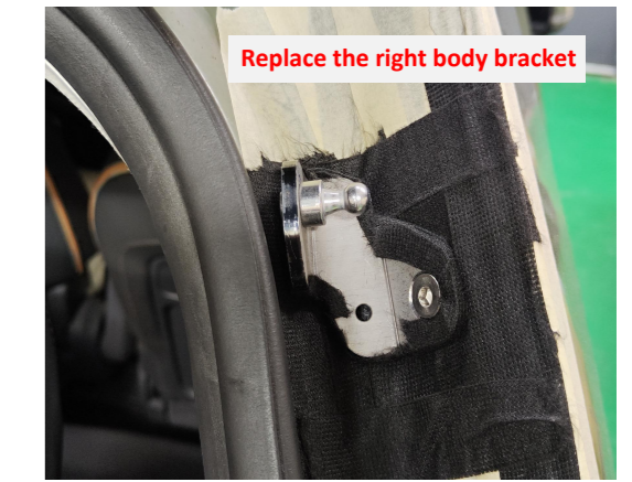
6. Replace the right body bracket.
