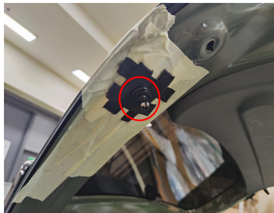
7. Replace the ball studs on both sides.
