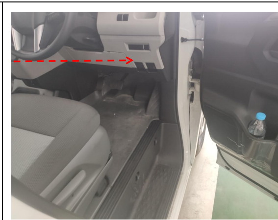
21. Thread the switch wiring harness from the front passenger side to the driver's position.
