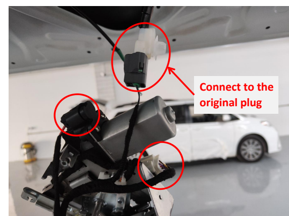
13. Connect the plugs of the lock signal harness to the power latch.
