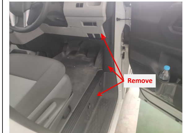
1. Remove the indicated trim panels and step board at the driver's area.
