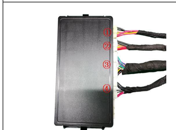
27. Insert the strut wiring harnesses ①②, lock signal harness ③, and power harness ④ into the ECU in sequence.
