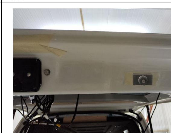
31. Install the hole opener and turn the nut to open the hole.
