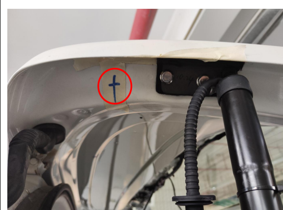
9. Drill a hole at the indicated location to allow the strut wiring harness to pass through. Both sides are the same.
