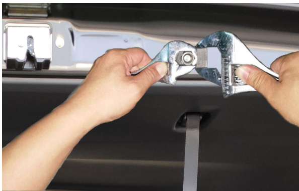
32. Use the wrenches to open the hole.
