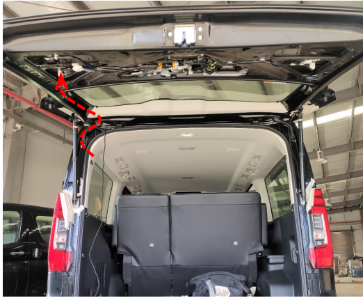
17. Thread the power harness to the tailgate (routing only, no plug or power connection).
