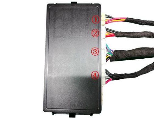
27. Insert the strut wiring harnesses ①②, lock signal harness ③, and power harness ④ into the ECU in sequence.
