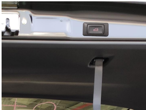
33. Install all the trim panels back and fit the added tailgate switch in.
