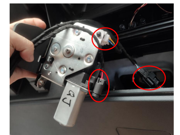
16. Connect the lock signal harness to the plugs of the power latch.
