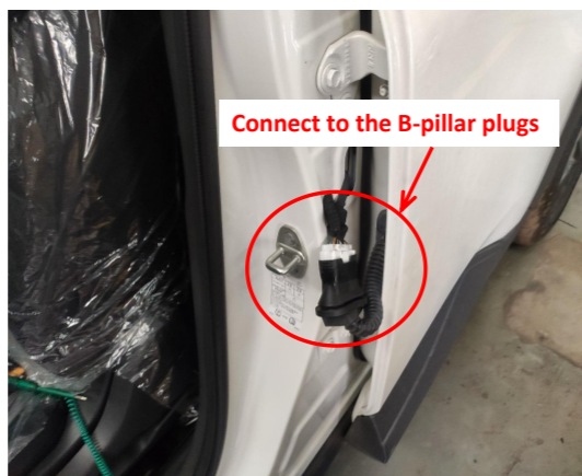
23. Connect the power harness to the indicated B-pillar plugs.
