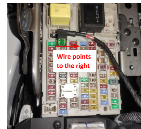
25. Plug the fuse tap into the fuse box. Pay attention to the direction.
