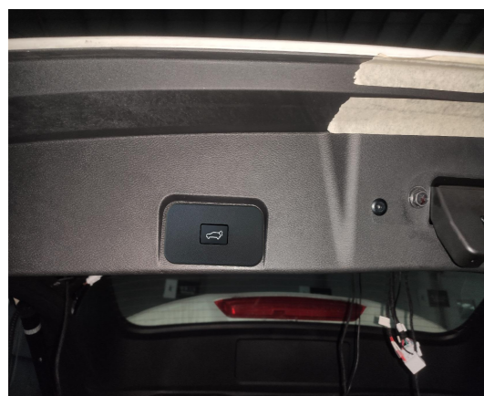
32. Install the added tailgate switch and reinstall all trim panels.
