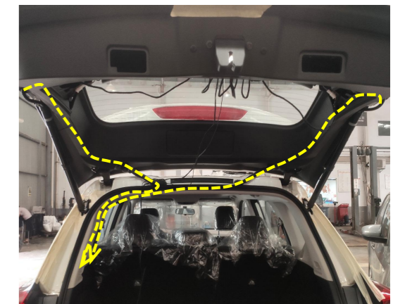
11. Route the left and right strut wiring harnesses to the left side of the trunk.
