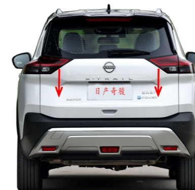
30. Press the added tailgate switch button to open and close the tailgate once for initializing the system, and then test each function of the electric tailgate.
