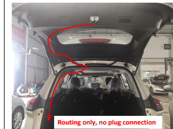
13. Route the lock signal harness to the left side of the trunk.
