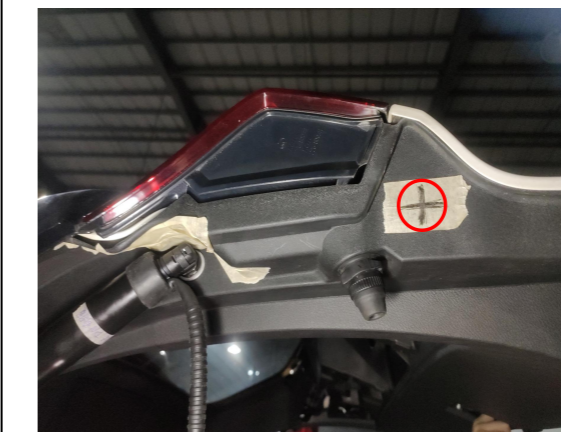
10. Drill a hole at the indicated position with the φ21mm drill bit to allow the strut wiring harness to pass through.
