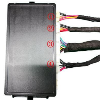
29. Insert the left and right strut wiring harnesses ①②, lock signal harness ③, and power harness ④ into the ECU in sequence.
