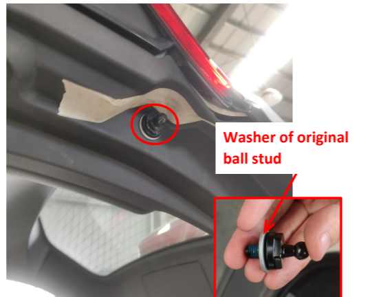
8. Replace the ball studs on both sides and place the original washers under them.
