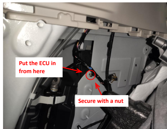
28. Install the ECU and secure it with nut.
