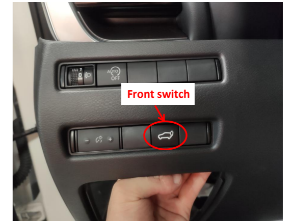
21. Remove the blank button from the indicated position and install the front switch button.
