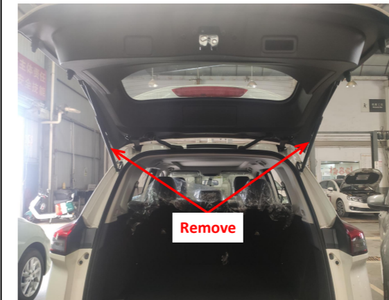
5. Remove the original gas struts.
