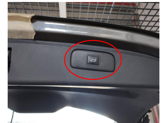
31. Reinstall all trim panels and fit the added tailgate switch in (remove the original small cover).
