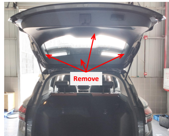
3. Remove the tailgate trim panels.
