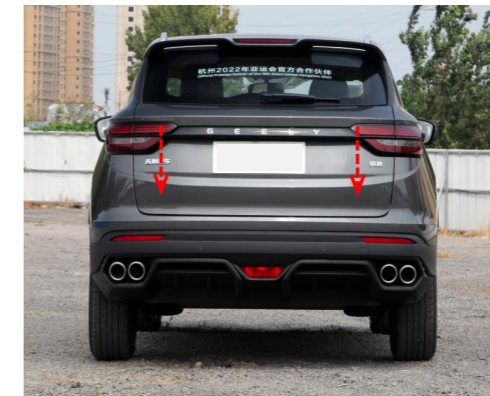
30. Press the added tailgate switch to close the tailgate once, the system completes initialization, and then test each function of the electric tailgate.
