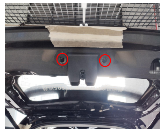
14. Remove the original latch.
