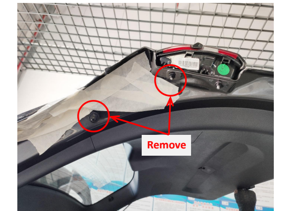
6. Remove the indicated ball stud and the nut on the tailgate lamp.
