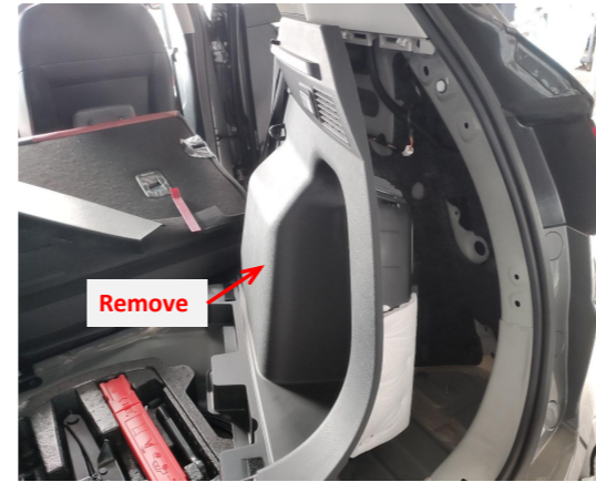
4. Take out the trunk floor mat and remove the trim panel on the right side of the trunk.
