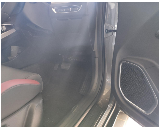
(Optional) Find an appropriate position at the driver's area, drill a \phi 21\text{mm} hole and install the added front switch.
