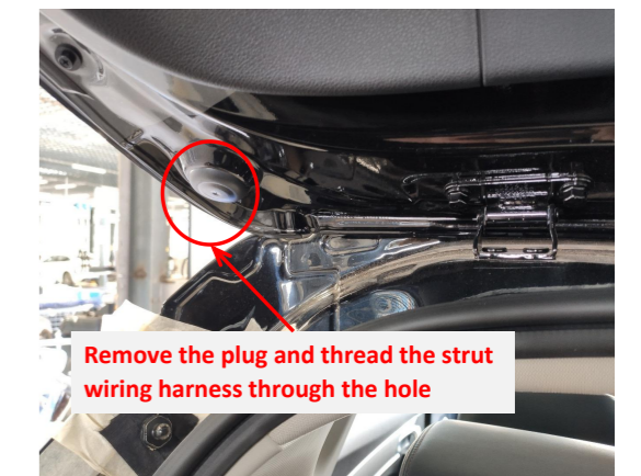
11. Thread the left and right strut wiring harnesses through the holes on both sides of the tailgate.
