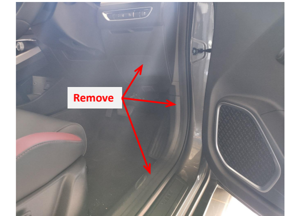
1. Remove the front right side trim panel, door sill panel and storage box.
