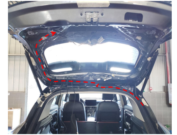
21. Thread power harness to the tailgate.
