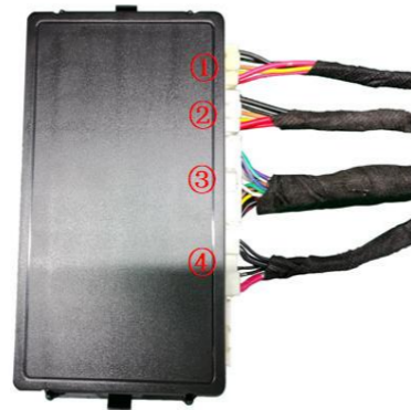
28. Insert the strut wire harness ①, lock signal harness ②, and power harness ④ into the ECU in sequence.
