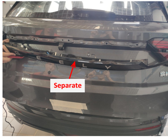
17. Separate the trim strip from the tailgate.
