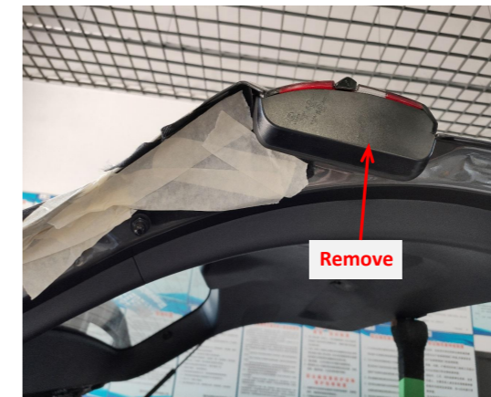
5. Remove the tailgate lamp covers on both sides.
