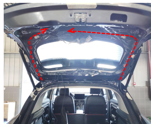
12. Route the strut wiring harnesses to the tailgate as indicated.
